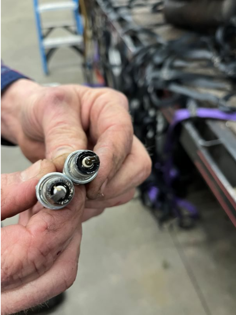
Figure 6 View of sparkplugs from the bottom of the cylinder.
