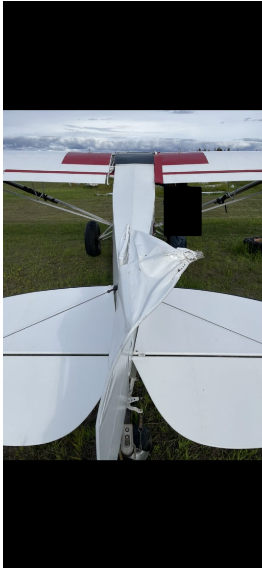
Photograph 1 - Aft view of damage to the airplane's tail. (Courtesy of owner)
