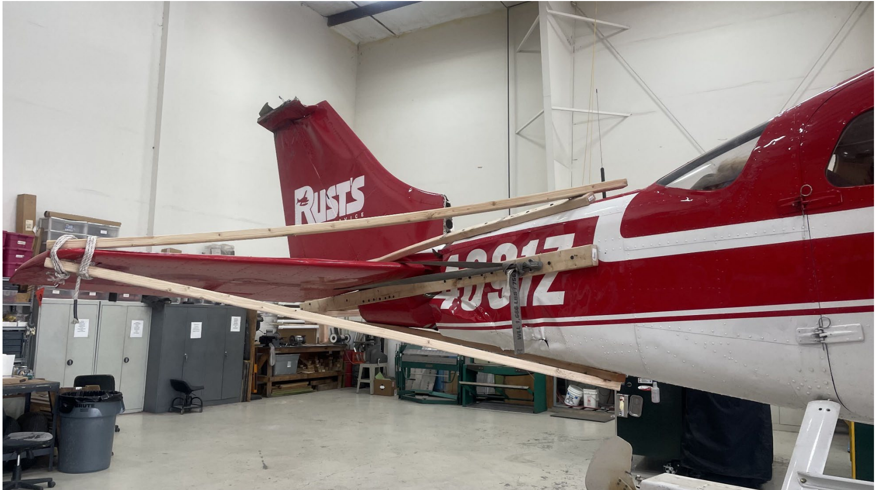
Photograph 1 - Damaged rudder and vertical stabilizer (Courtesy of Operator)
