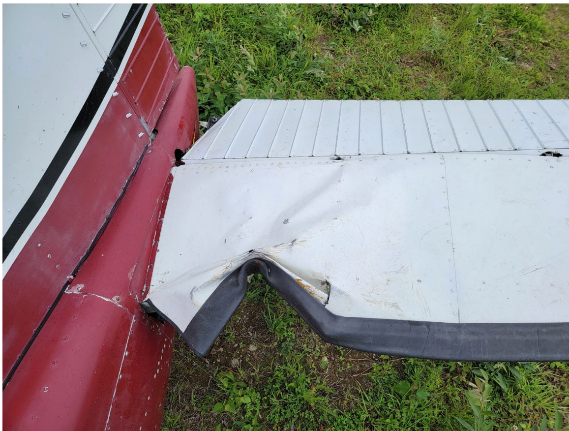
Photograph 2 - Damaged left horizontal stabilizer (Courtesy of NTSB Investigator)
