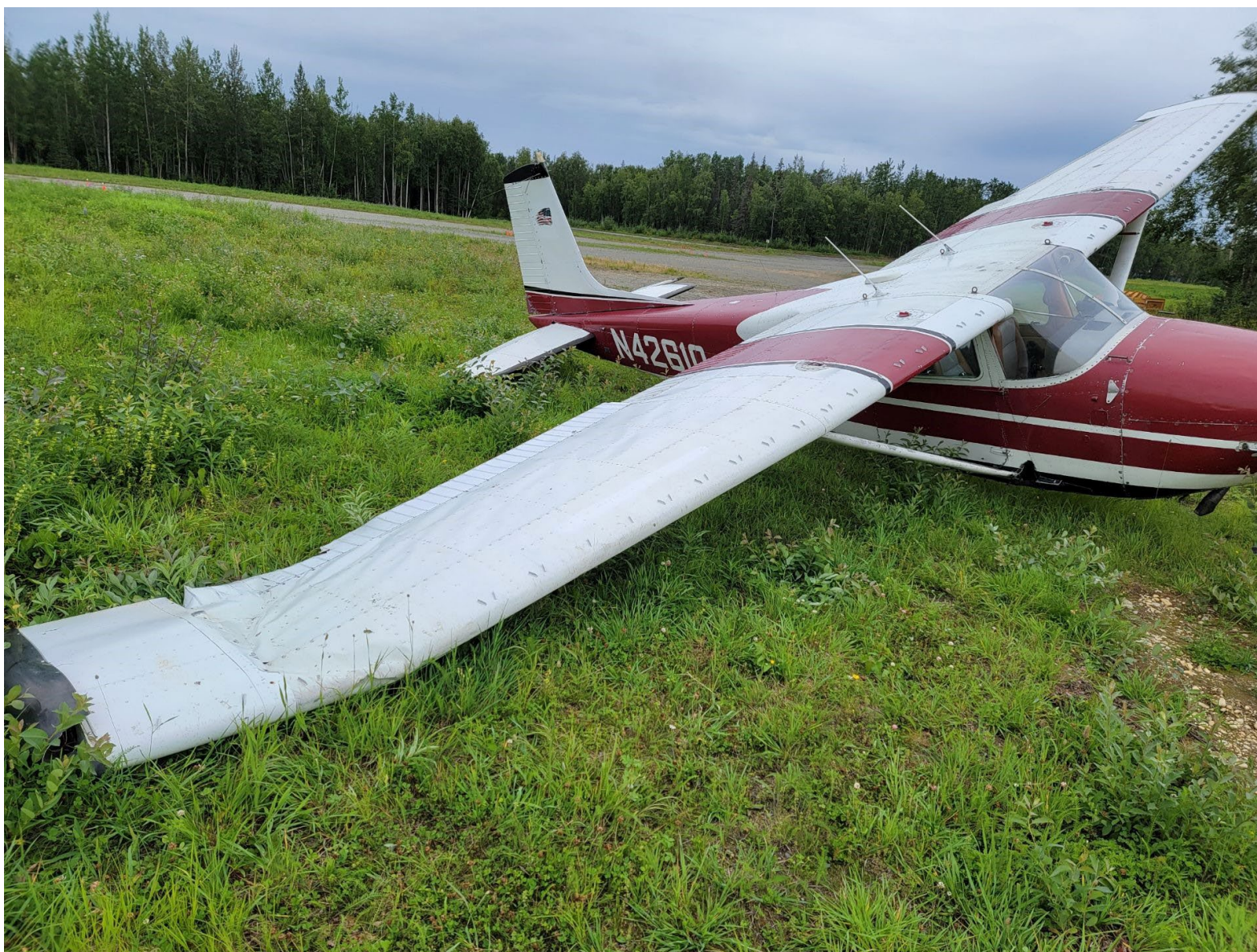
Photograph 1 - Damaged right wing (Courtesy of NTSB Investigator)
