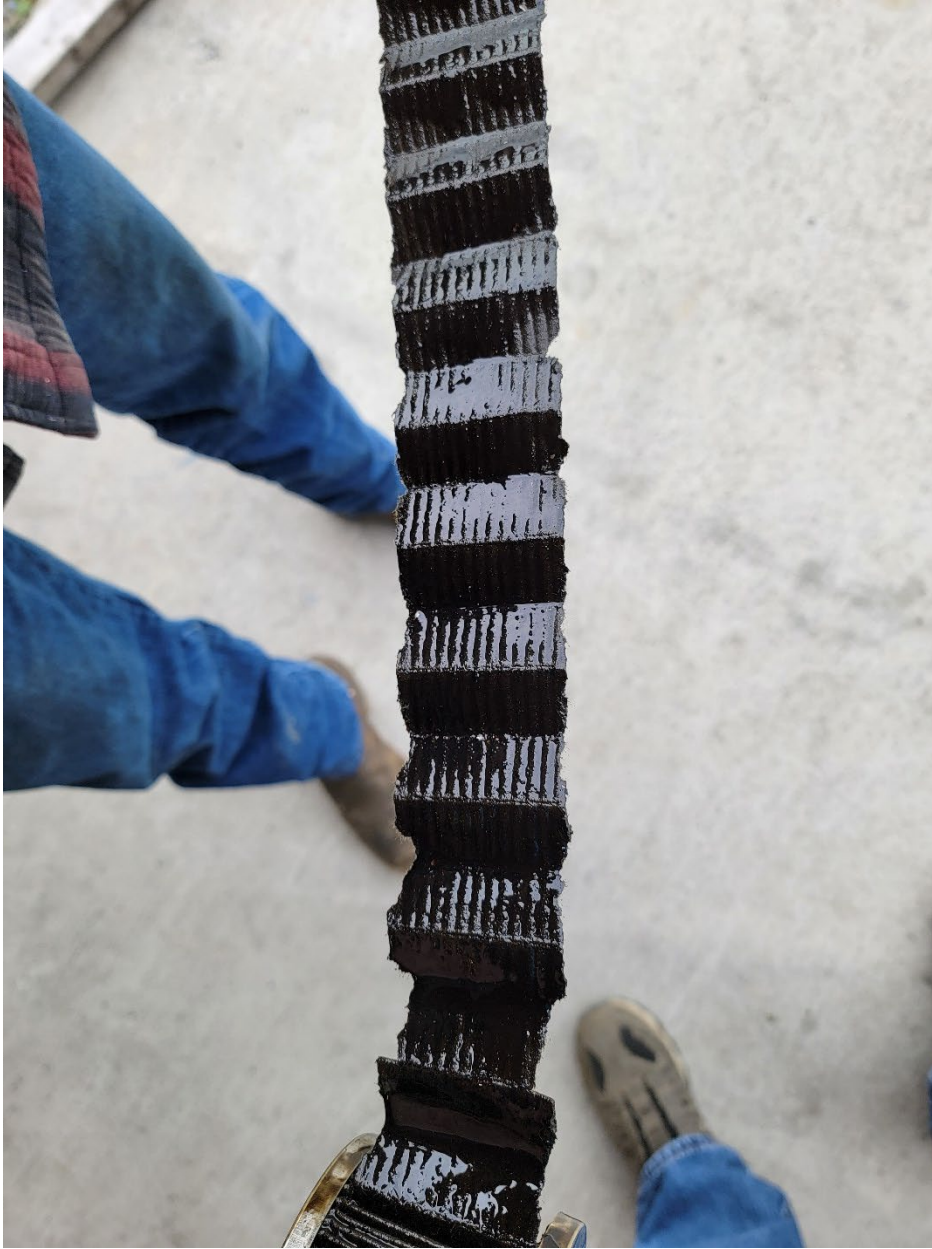
Figure 3. View of oil filter.
