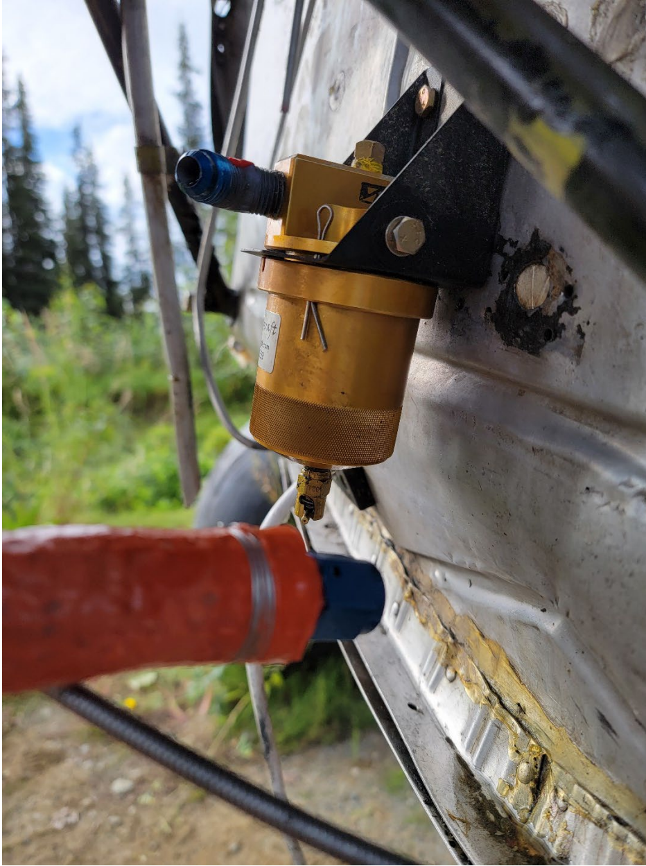
Figure 4. View of gascolator.
