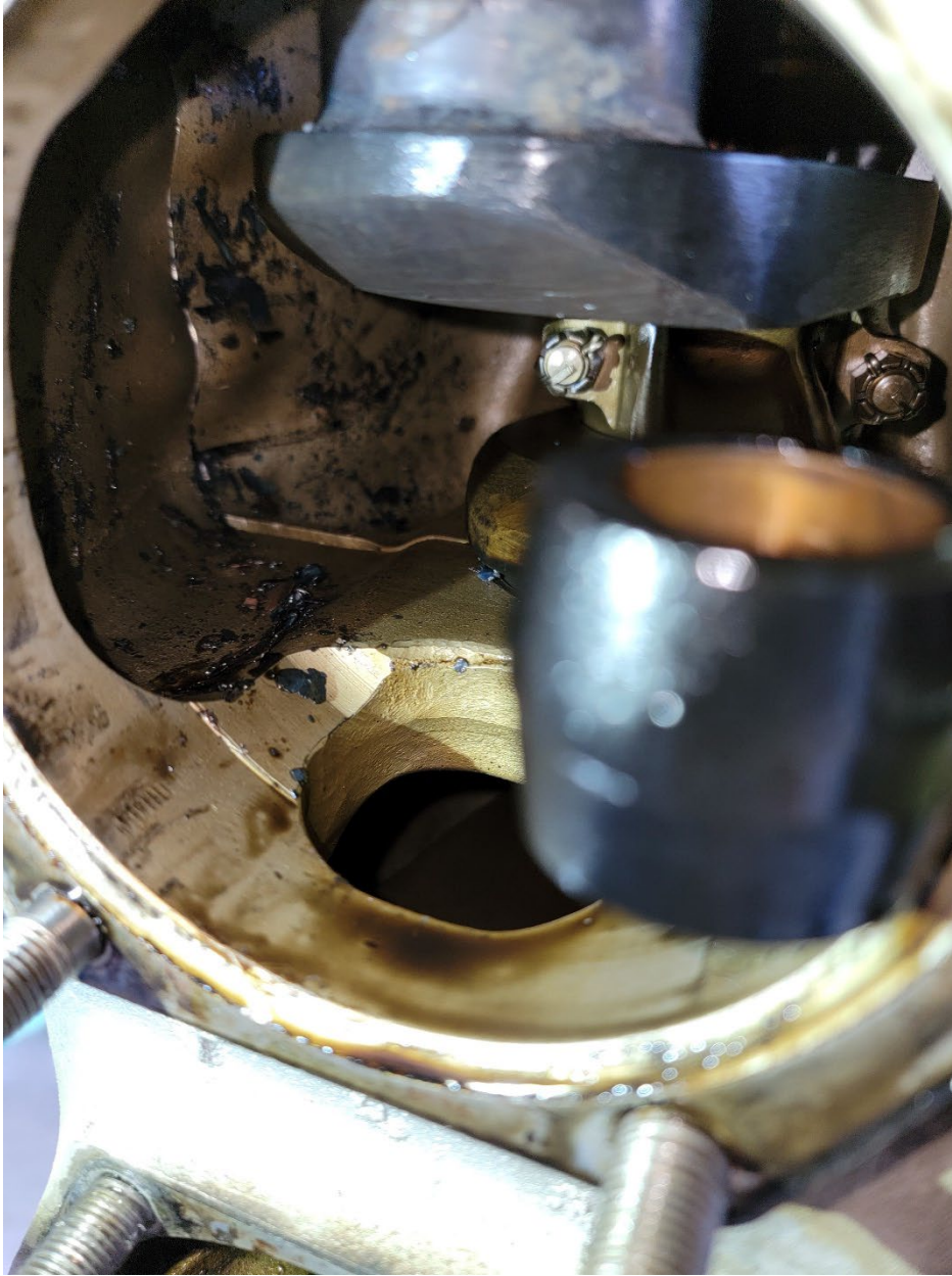
Figure 9. View looking inside the engine case and fragments of a main bearing.
