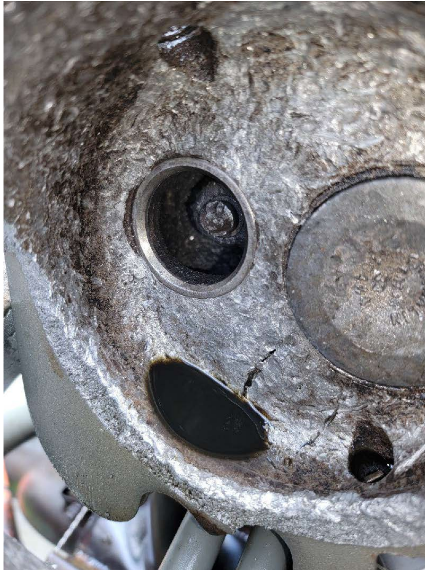
Photograph 2 - View inside the No. 1 cylinder after removal from engine, note the remaining portion of the exhaust valve stem.
