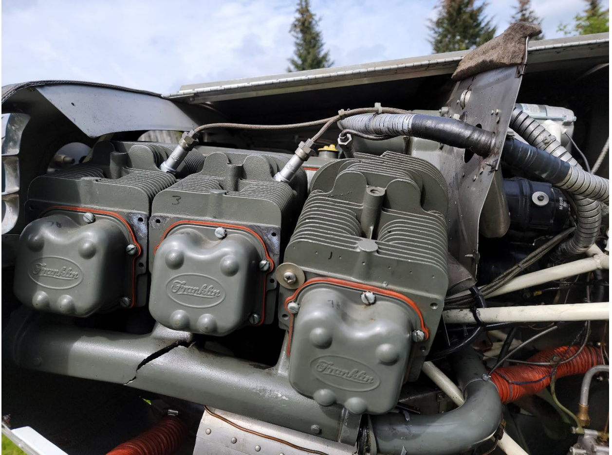
Figure 1 View of the left side of the engine, note cylinder No. 1 partially separated.
