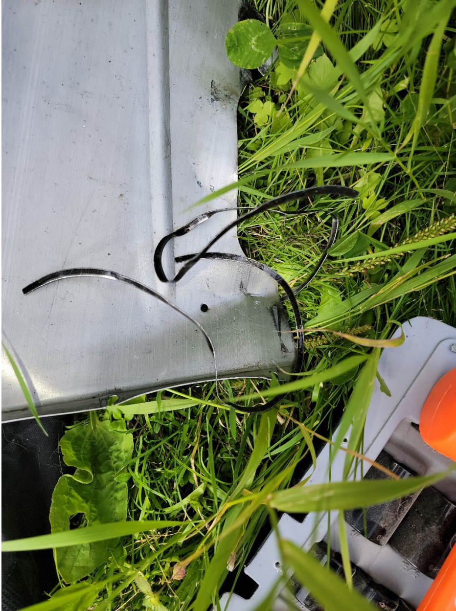
Figure 5 View of the No. 1 cylinder piston rings after being removed from the engine.
