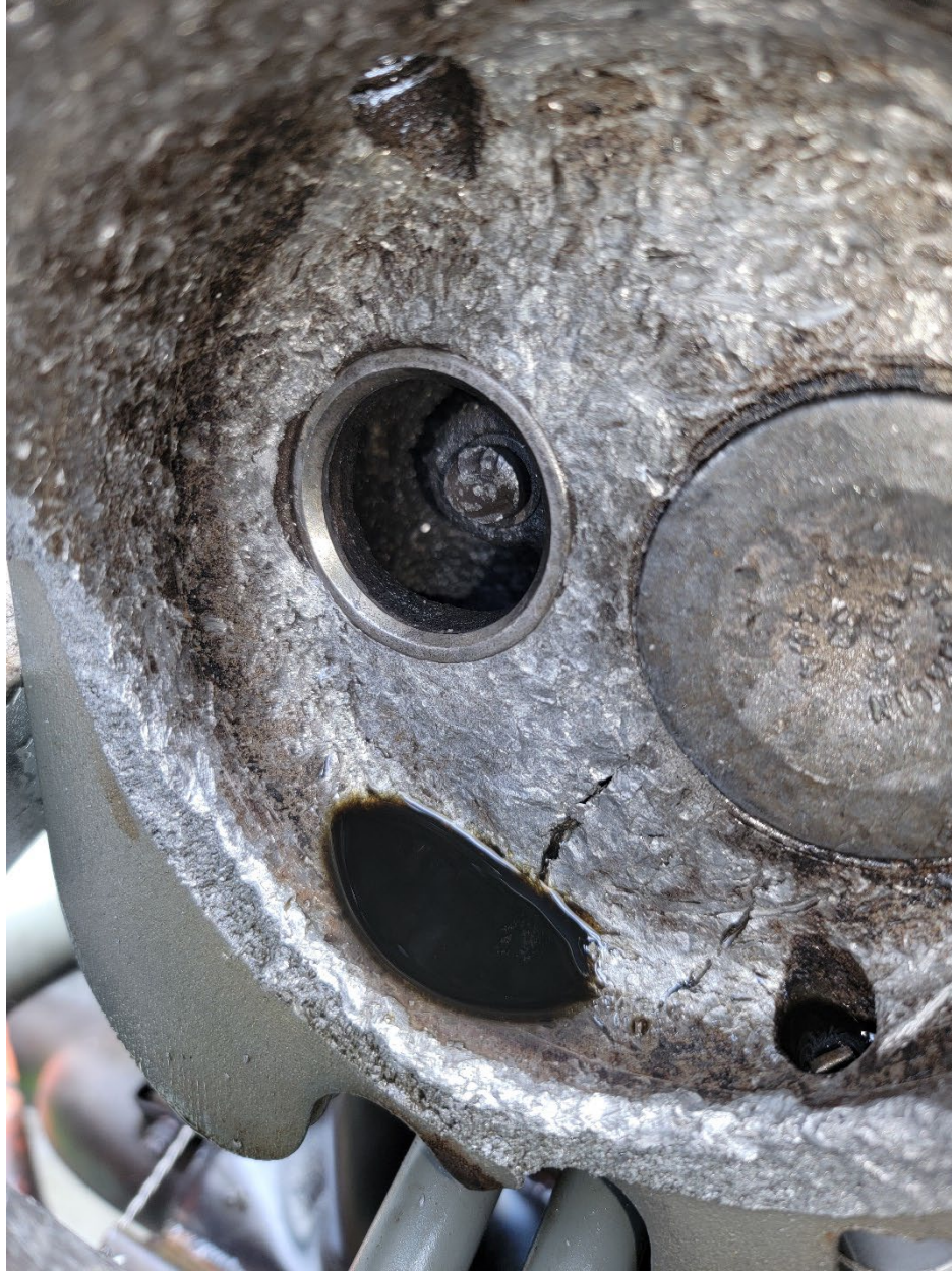
Figure 6 View inside the No. 1 cylinder after removal from engine, note the remaining portion of the exhaust valve stem.
