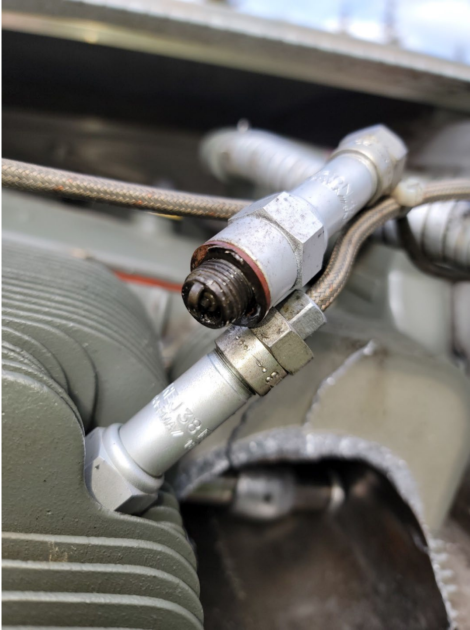
Figure 4 No. 1 top sparkplug, the bottom sparkplug remained loosely attached to the cylinder.
