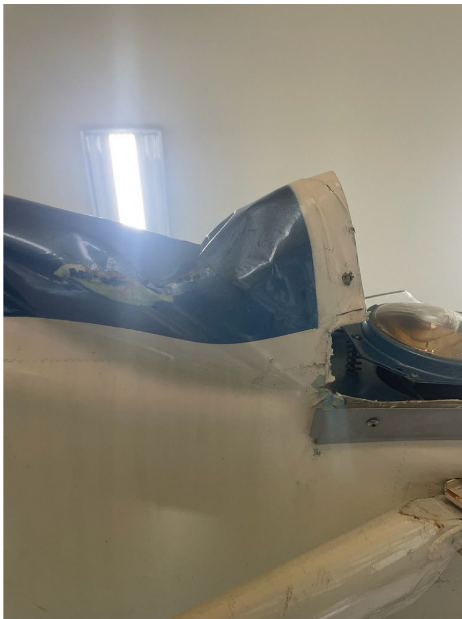
Photo 3 – Right-wing leading-edge damage near landing light. Photo provided by owner.
