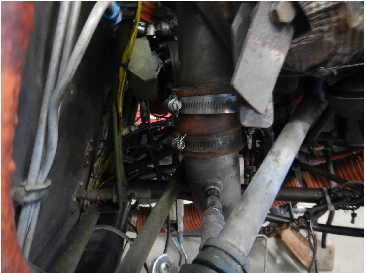
Figure 5 Hose connection to the engine turbo.
