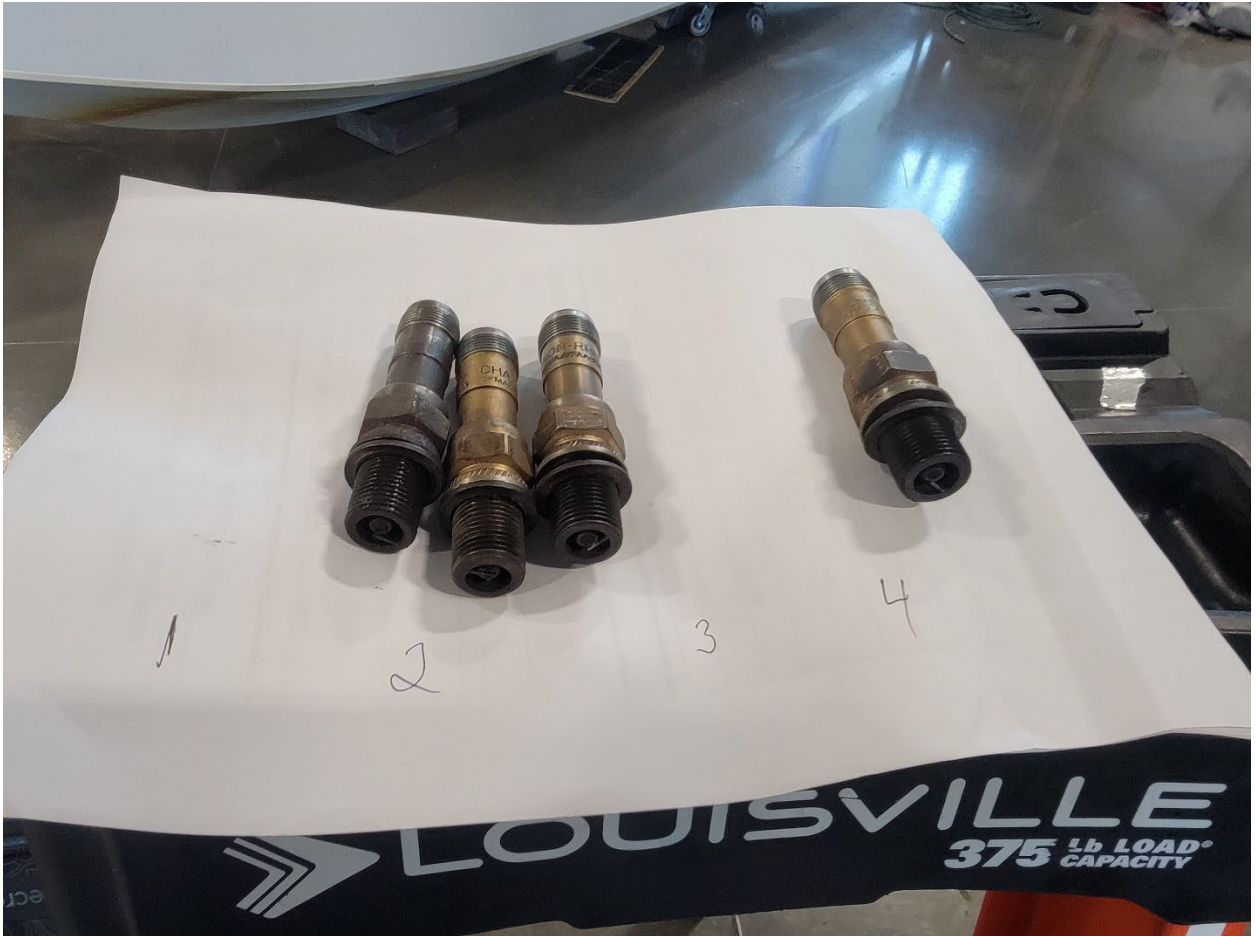
Figure 4 Spark plugs removed from the bottom side of the engine.
