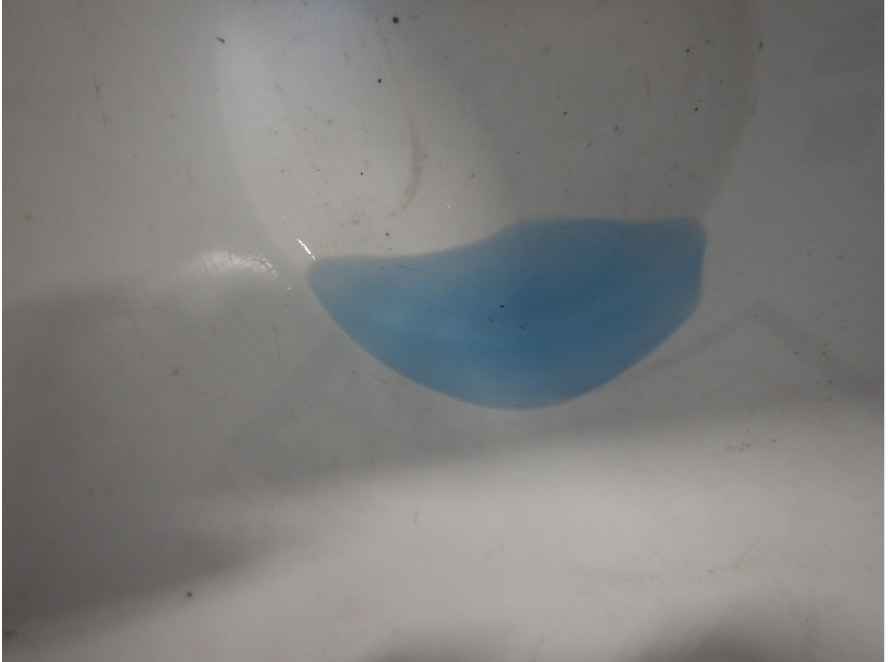
Figure 3 Fuel removed from gascolator
