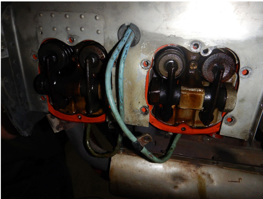
Figure 8 Left side of engine, valve covers removed.
