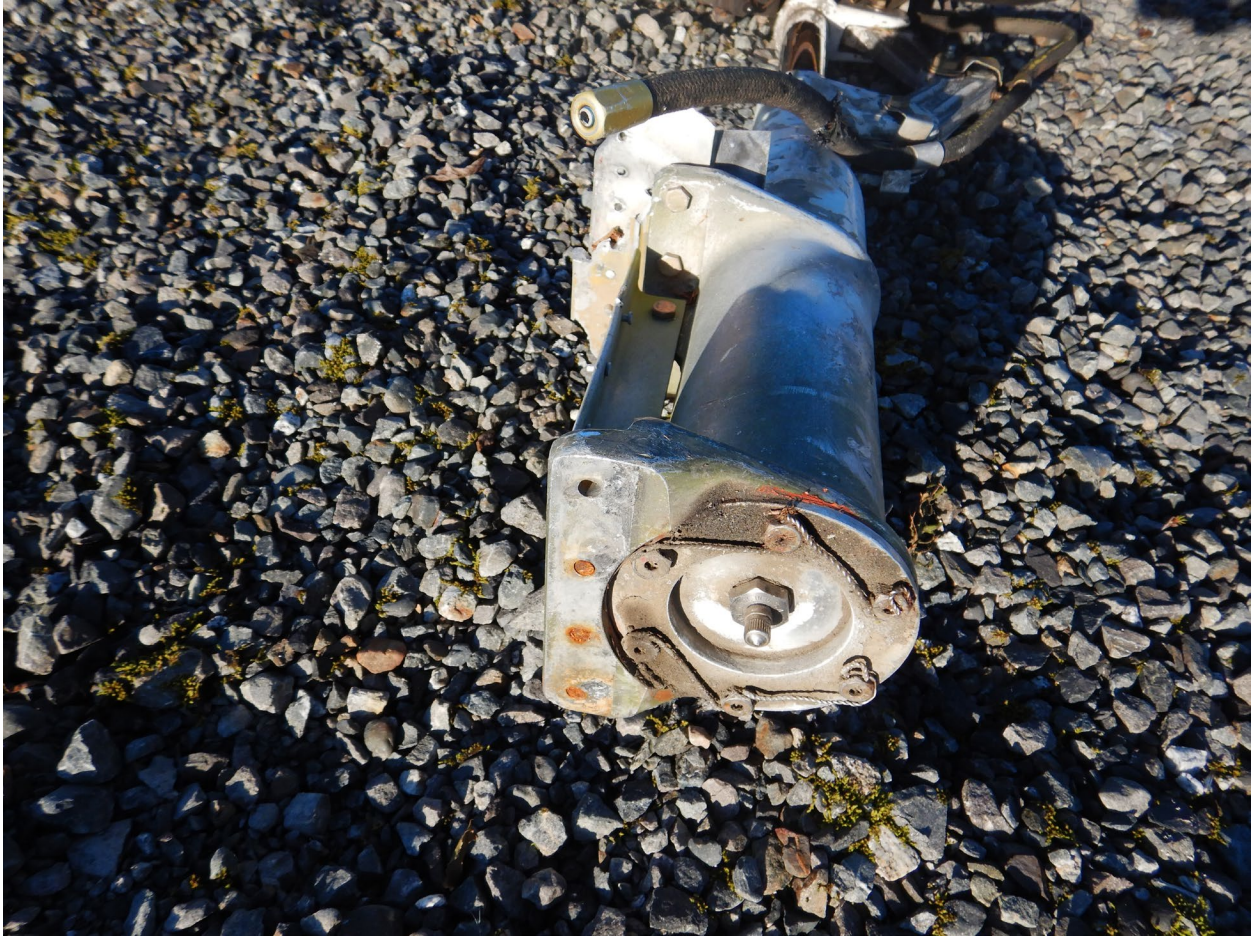
Figure 29. View of the right landing gear assembly looking down from the attachment point to the tire.
