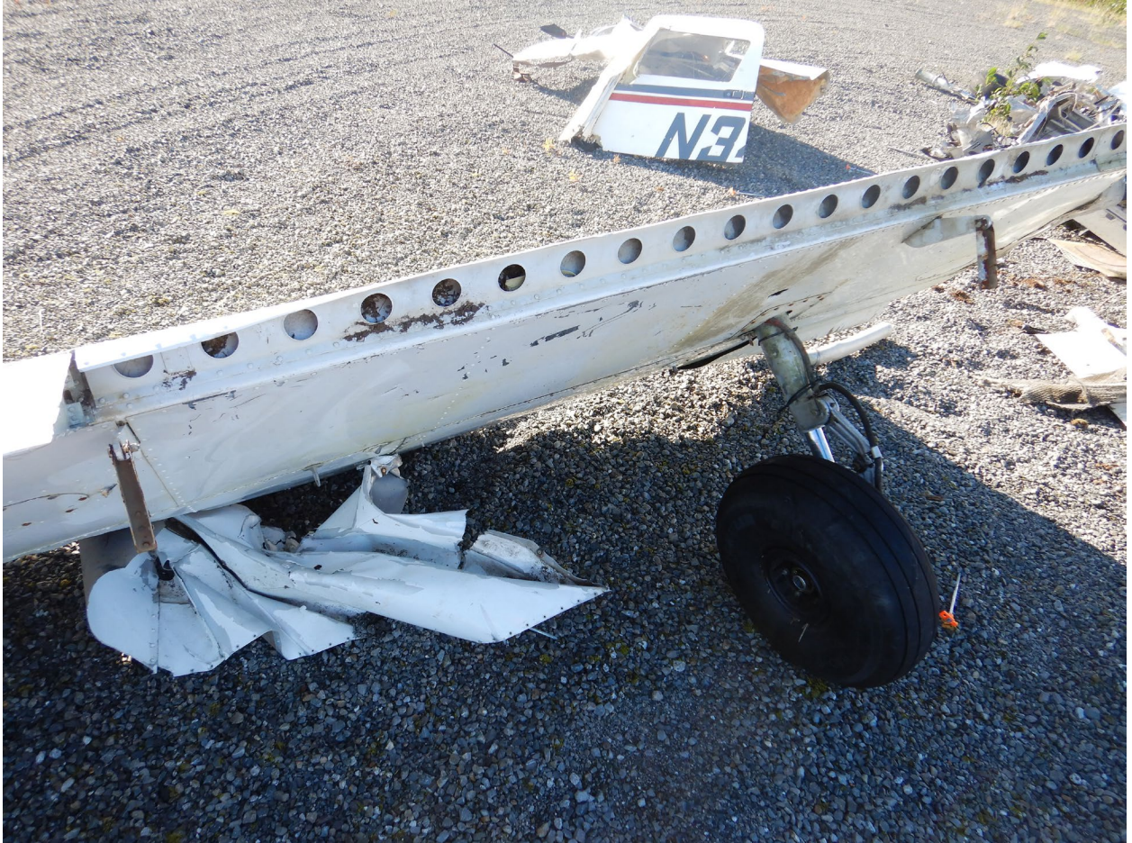
Figure 23. View of left wing from the rear looking at the flap attachment area.
