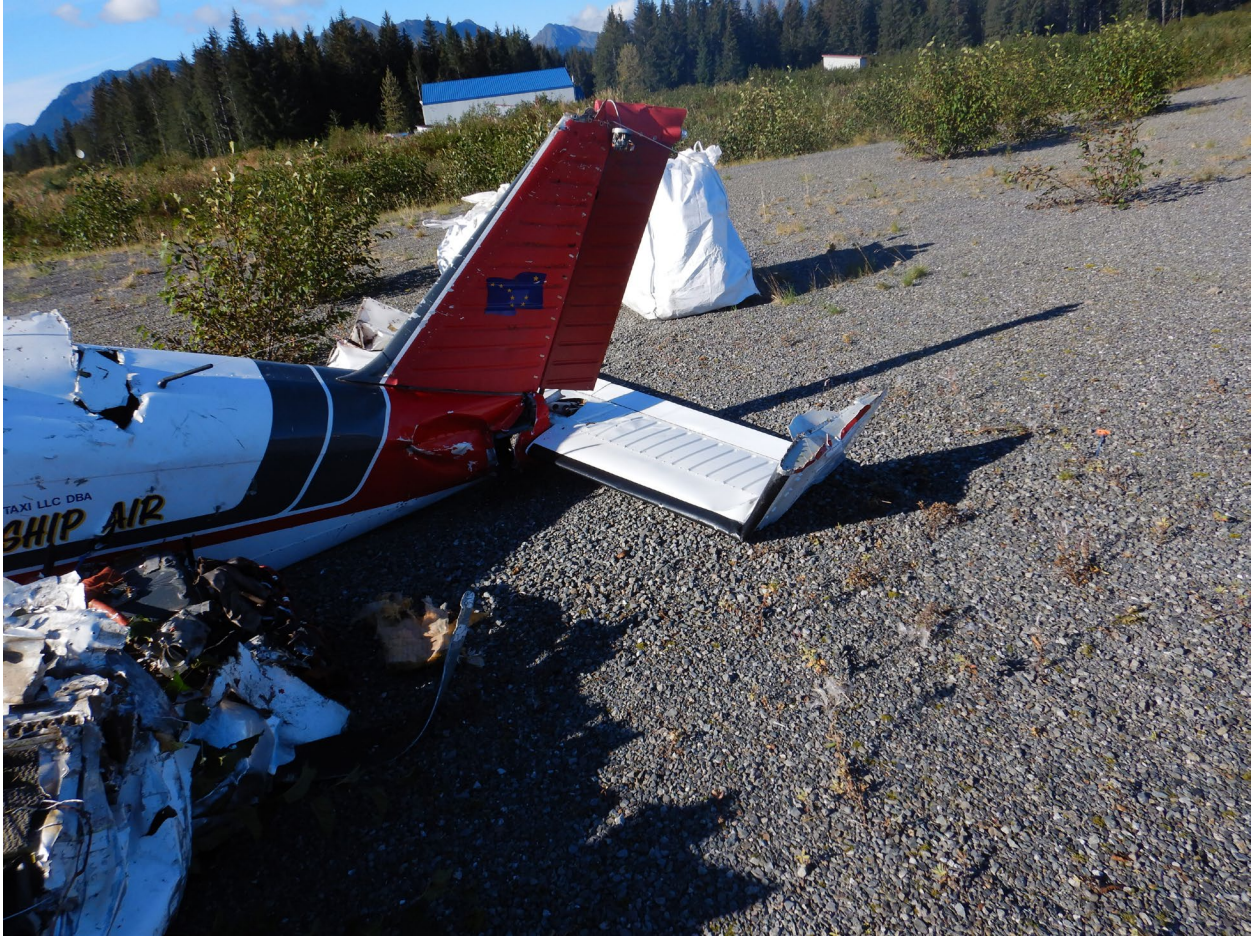
Figure 10. View of the left side of the empennage and damage to the left side of the elevator.
