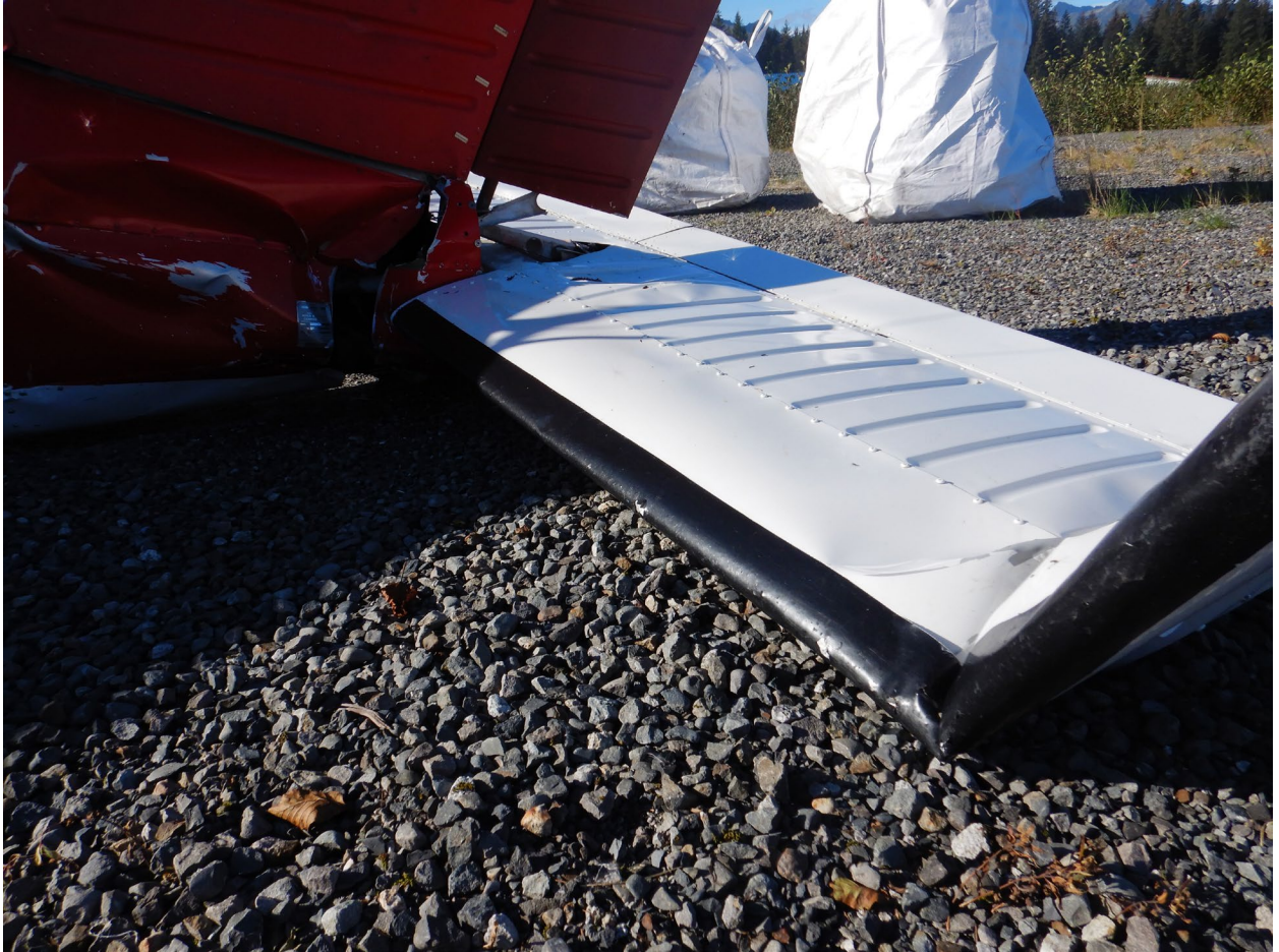
Figure 14. View of leading edge of the left side of the elevator.
