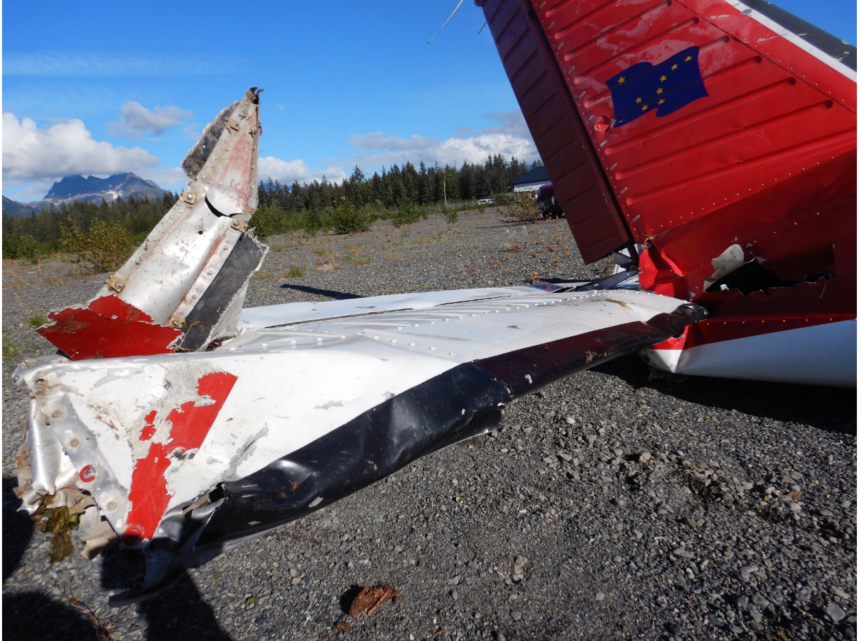
Figure 13. View of damage to leading edge of the right side of the elevator.
