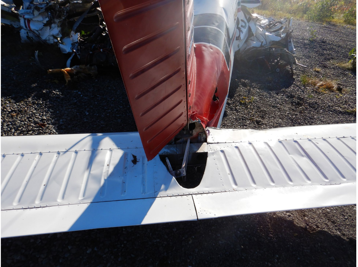
Figure 15. View of the trim tab and upper portion of the elevator.
