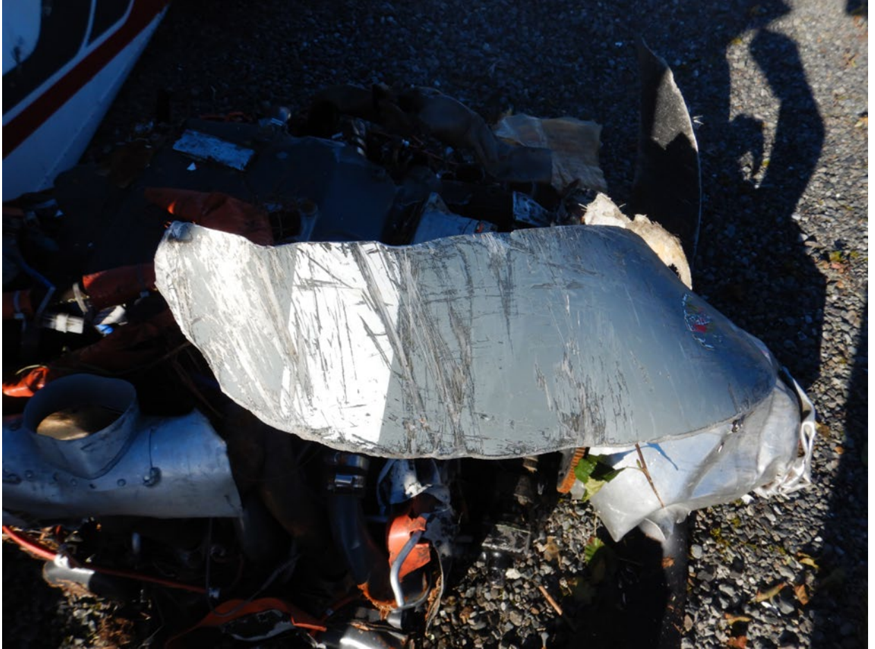
Figure 46. View of engine propeller.
