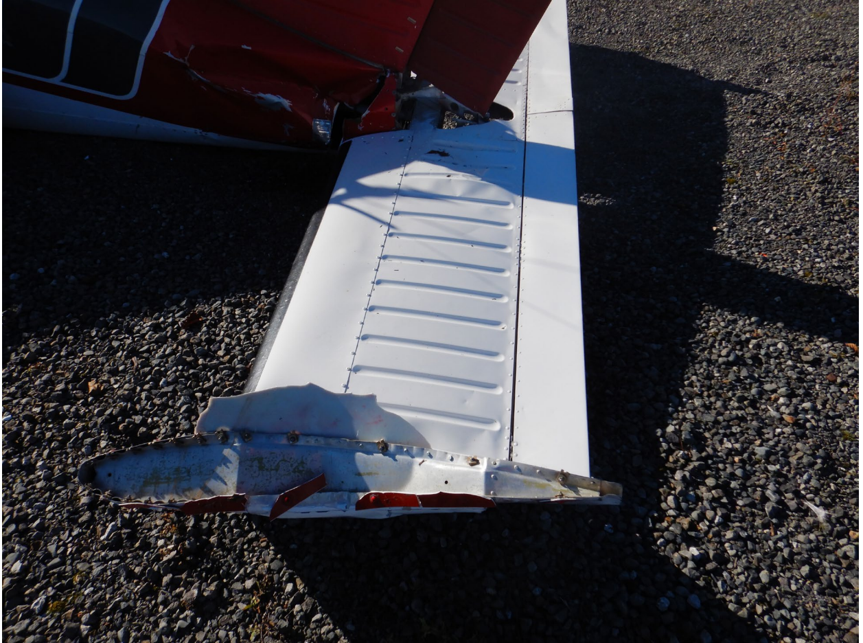
Figure 12. View of damage to left side of the elevator.
