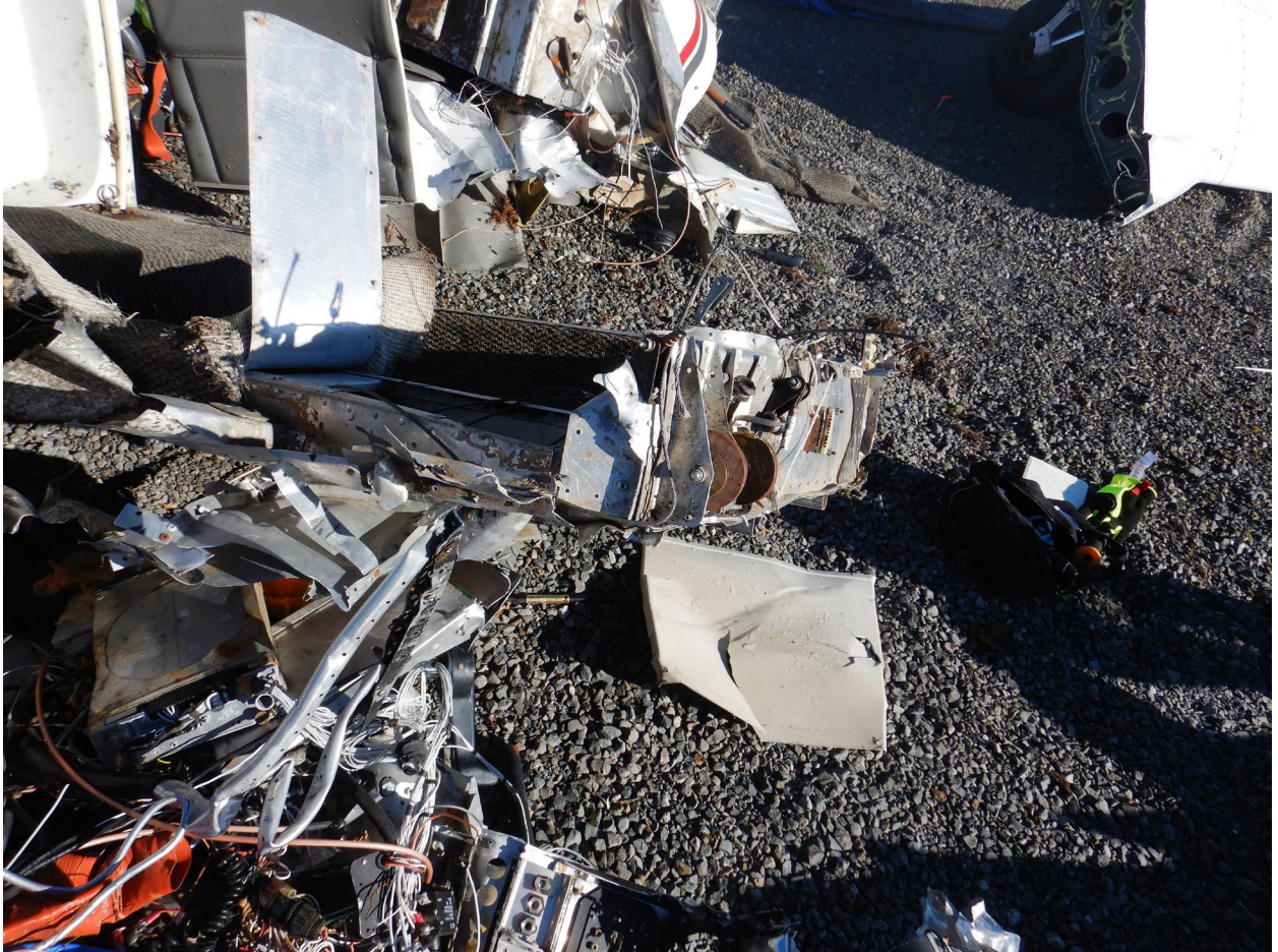
Figure 20. Side view of the flight control cables about 5.5 ft from the baggage compartment wall.
