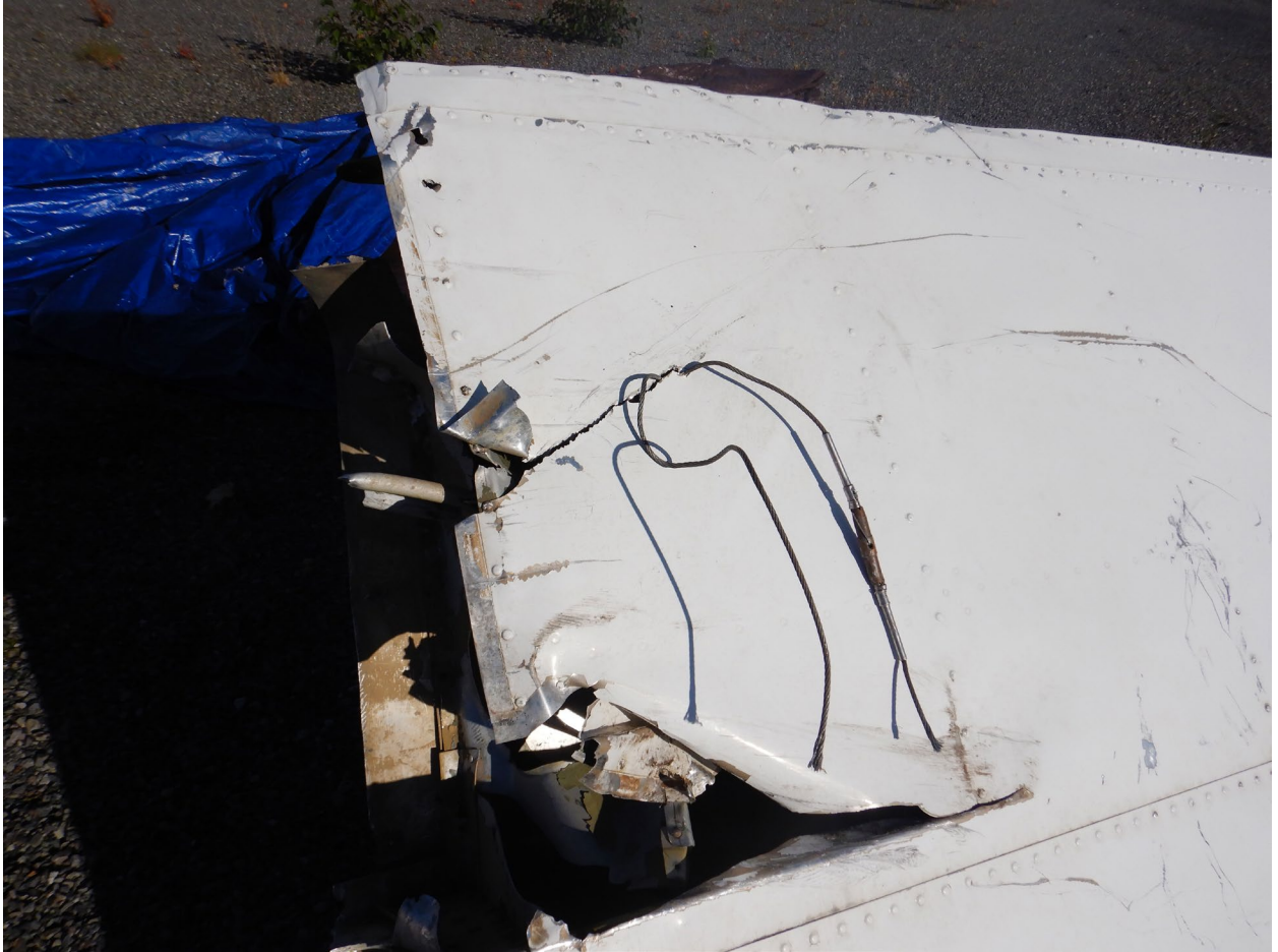
Figure 24. View of left wing at the root. Flight control cables pulled through upper wing surface.
