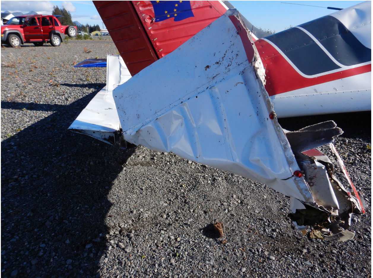
Figure 11. View of the damage to the right side of the elevator.
