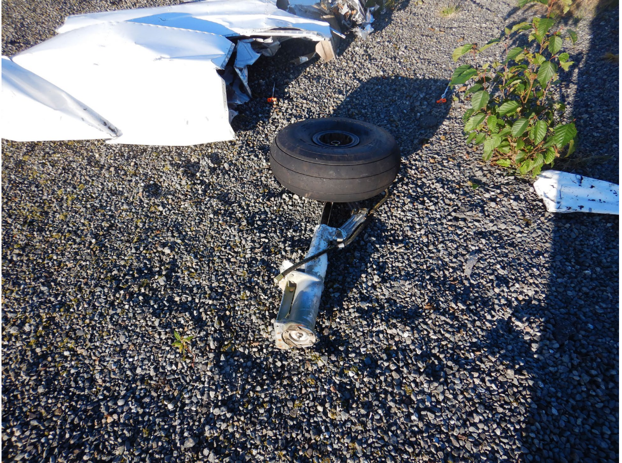
Figure 28. View of right landing gear assembly.
