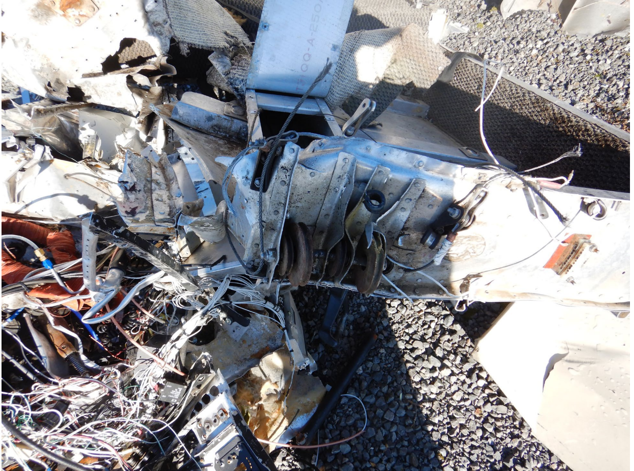
Figure 19. View of flight control cable breaks along the floor about 5.5 ft from the baggage compartment wall.
