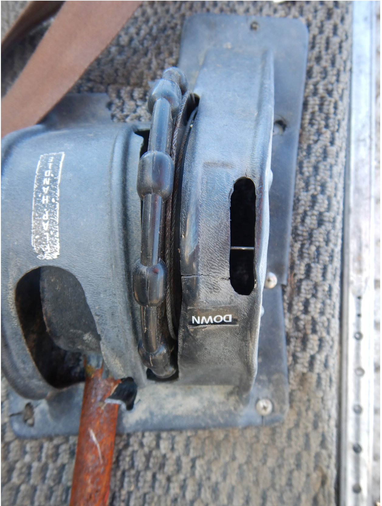
Figure 33. View of flap handle and trim setting.
