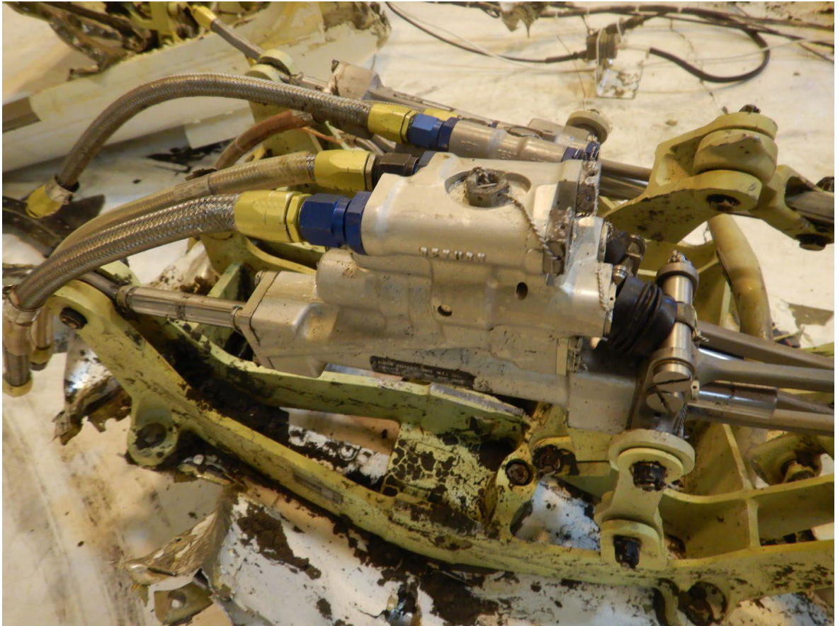
Figure 44 Flight control servo.
