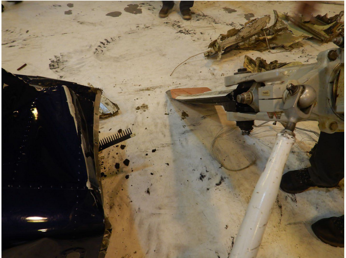
Figure 57 View of attachment point of intact main rotor blade.
