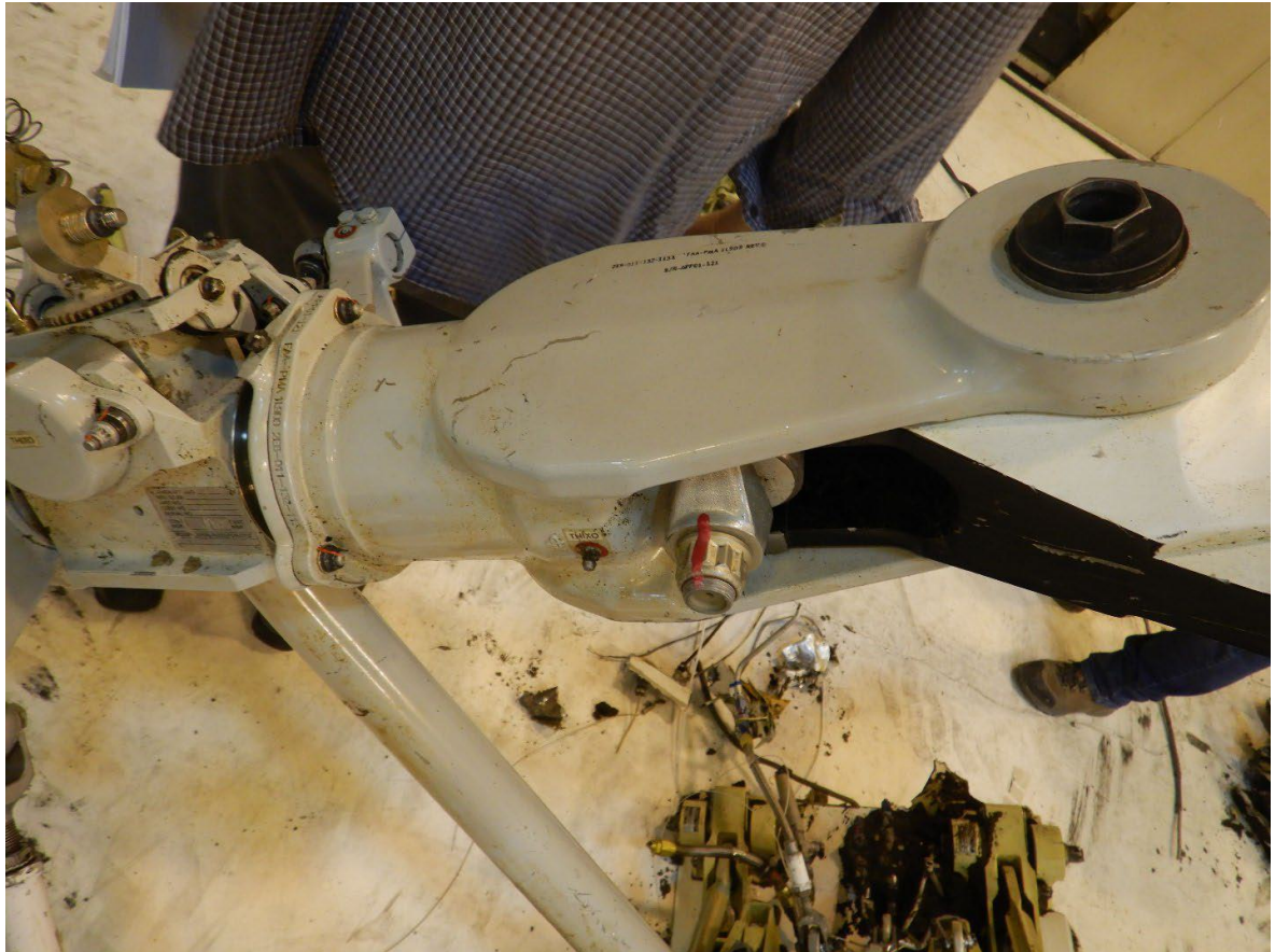
Figure 60 Main rotor hub attachment to non-intact rotor blade.
