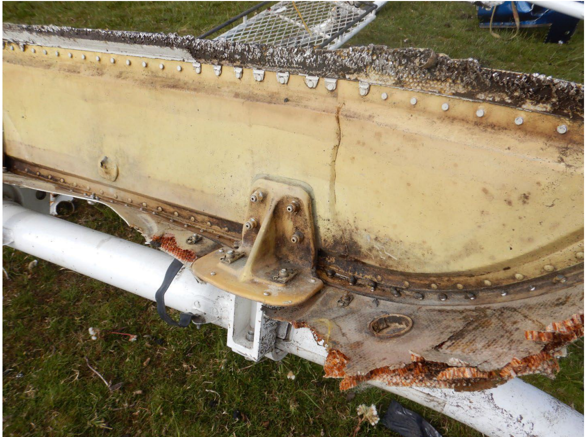
Figure 37 Rear view of the rear landing gear right attachment point.
