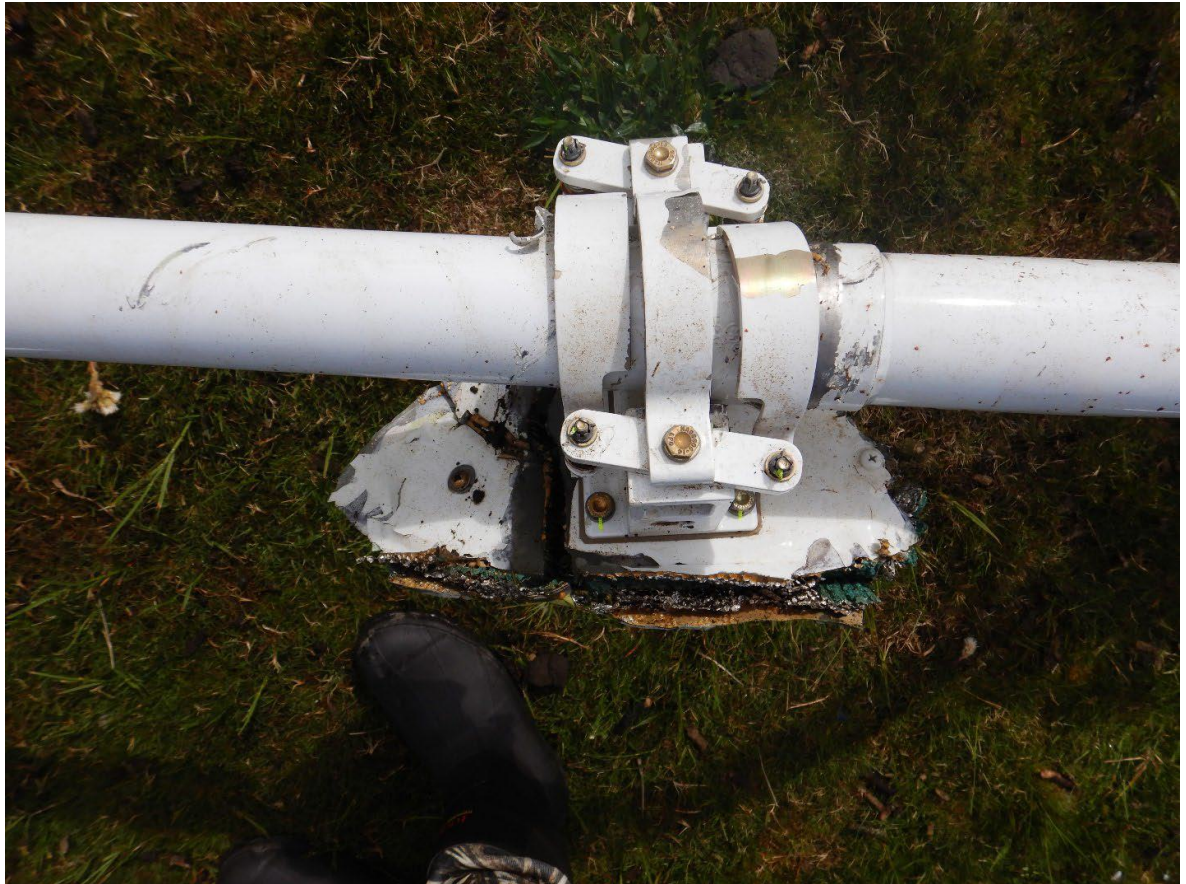
Figure 35 Front crossover tube of the landing gear's right attachment point.
