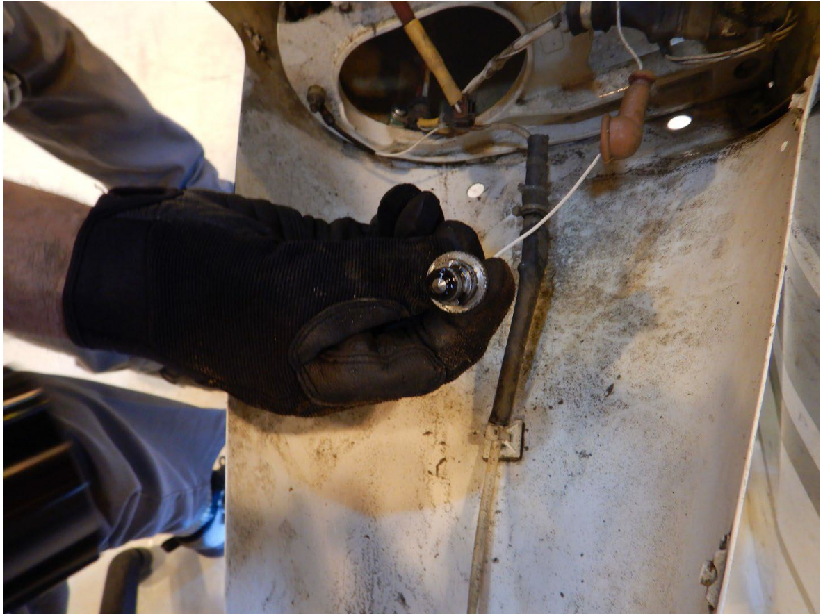
Figure 25 View of tail rotor chip detector.
