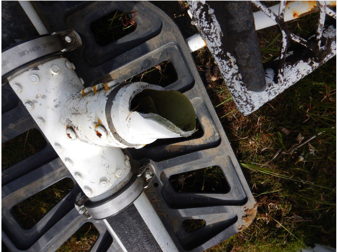
Figure 39 View of the fracture between the left landing gear skid and the rear crossover tube.
