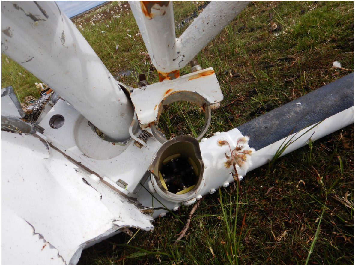
Figure 40 View of the fracture between the right landing gear skid and the front crossover tube.
