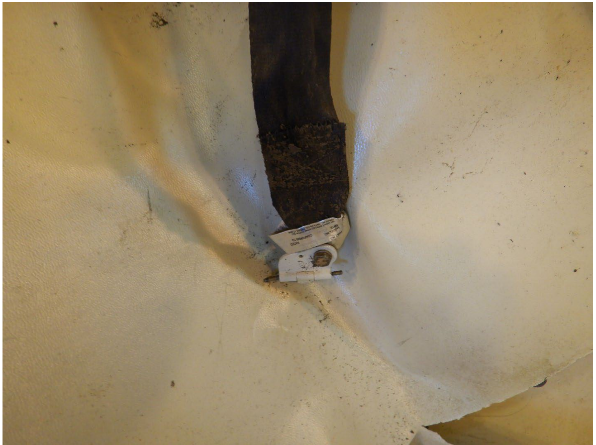
Figure 48 Broken seat belt attachment.
