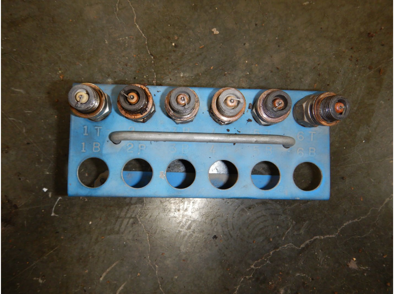
Figure 5. Top row of spark plugs removed from engine.
