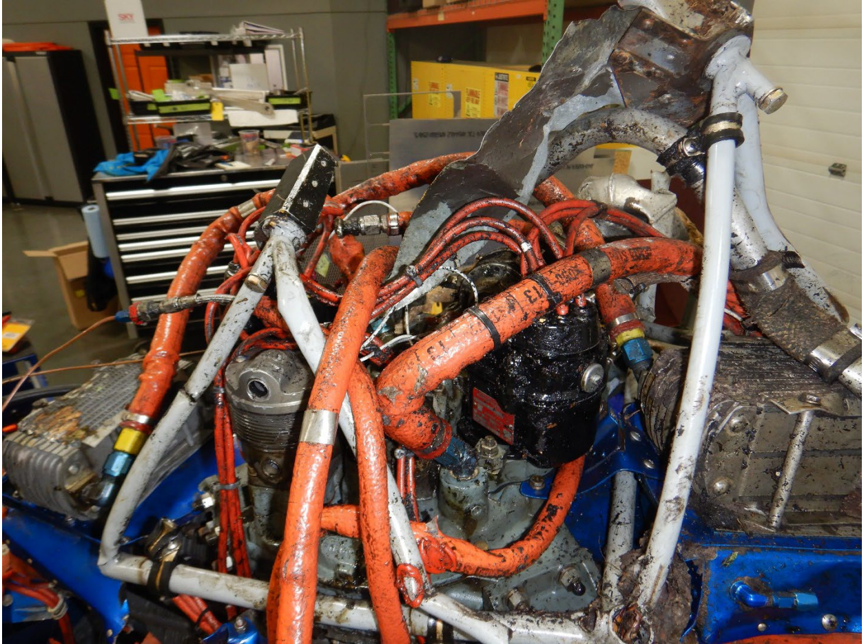
Figure 4. Accessory gear box on rear of engine.
