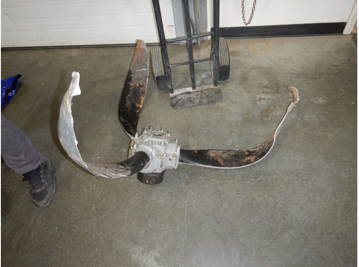
Figure 8. Propeller assembly after removal from engine.
