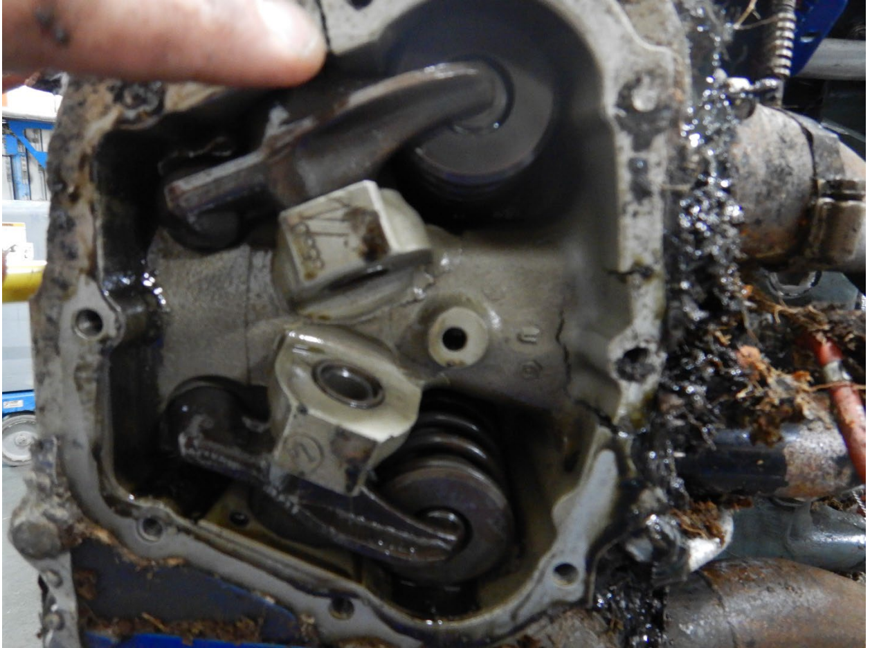
Figure 6. View of cracks in cylinder.
