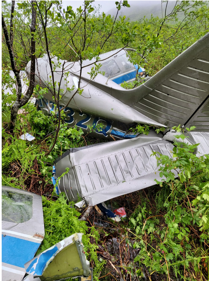
Photograph 4 - Aft view of the accident airplane at the accident site. (Courtesy of NTSB)
