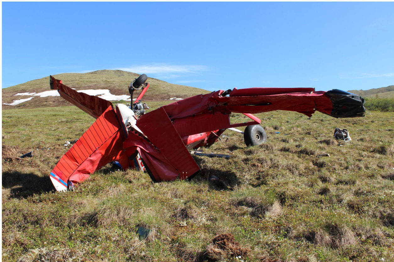
Photograph 3 - Rear view of the wreckage and the left horizontal stabilizer.
