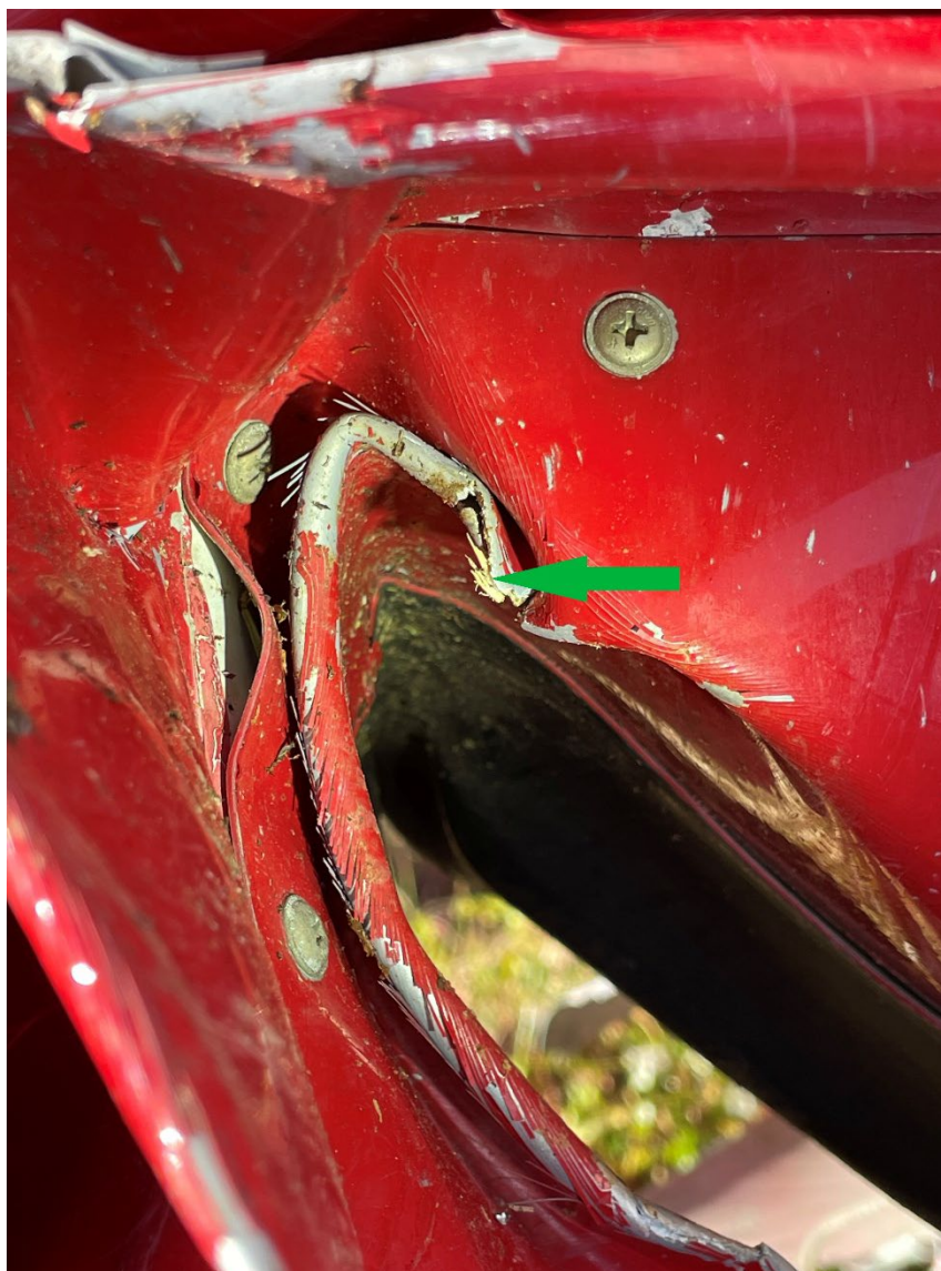
Photograph 10 - View of tree sap and embedded tree fibers in the leading edge of the horizontal stabilizer.
