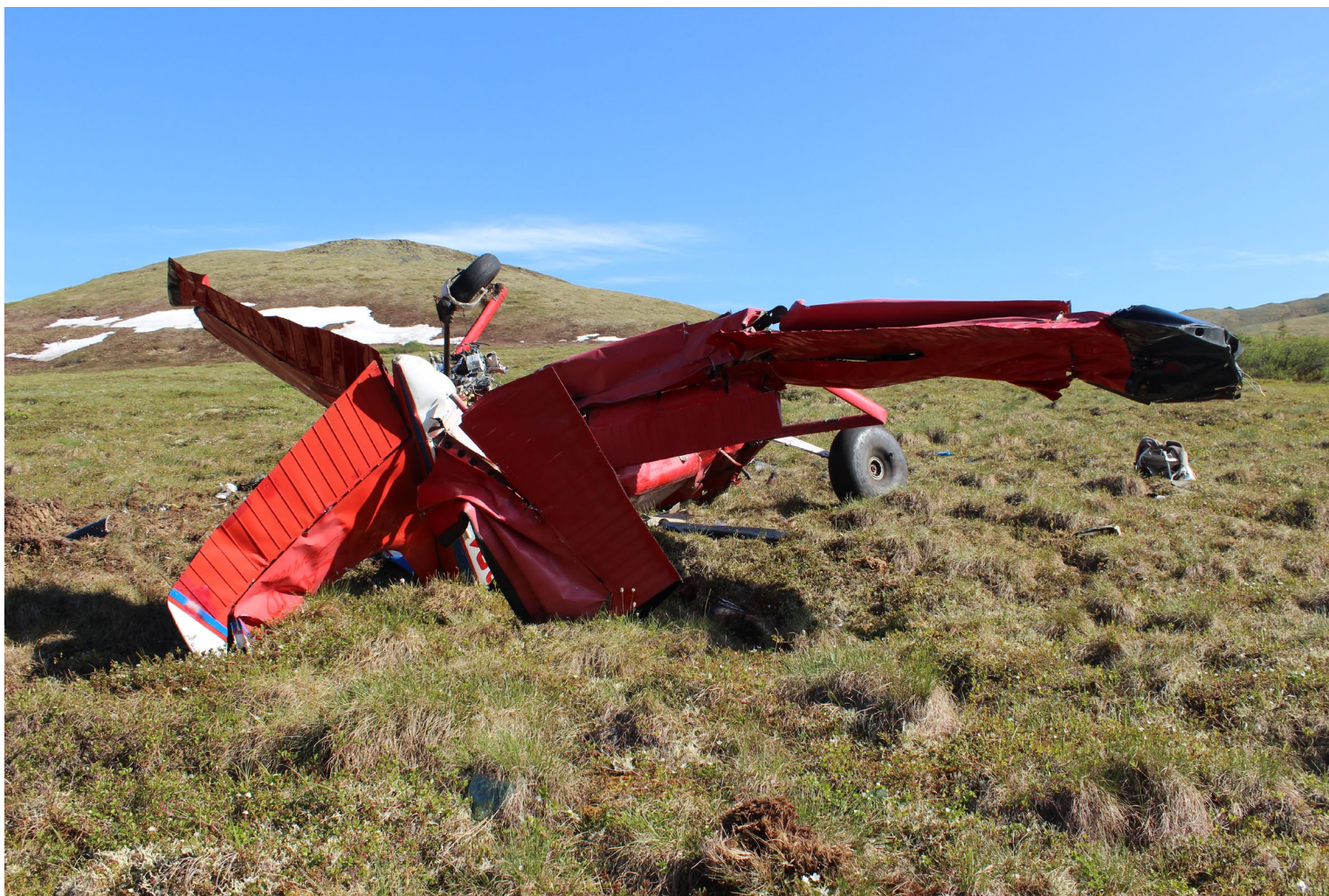
Photograph 6 - Rear view of the wreckage and the left horizontal stabilizer.
