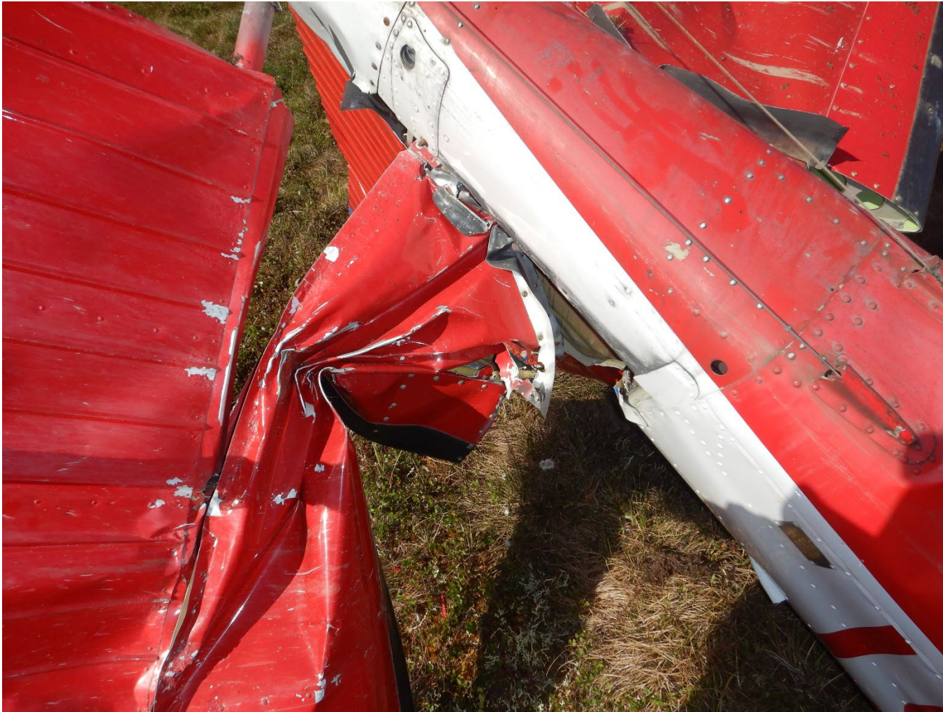
Photograph 8 - View of the leading edge damage to the left horizontal stabilizer (Courtesy of Textron Aviation)
