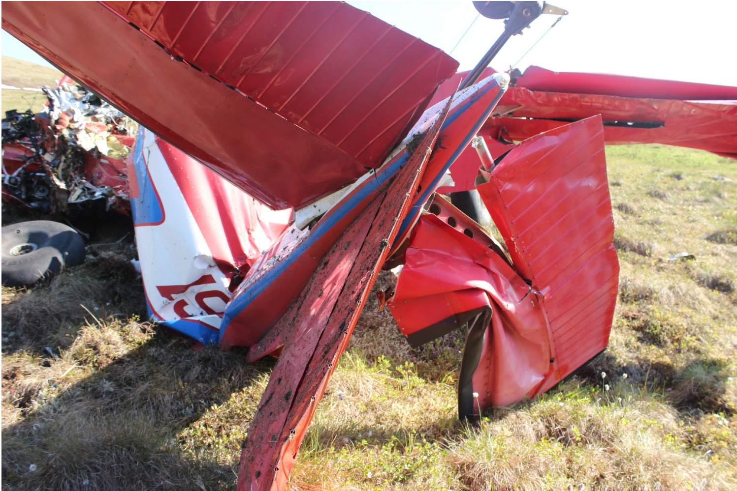
Photograph 7 - View of the horizontal stabilizers and rudder.
