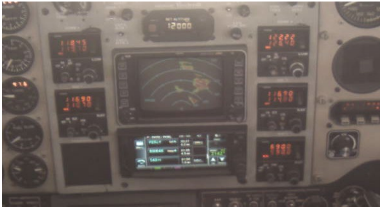
Figure 5. Image showing the Collins MFD working on a previous flight. The time of this image being taken could not be determined.
