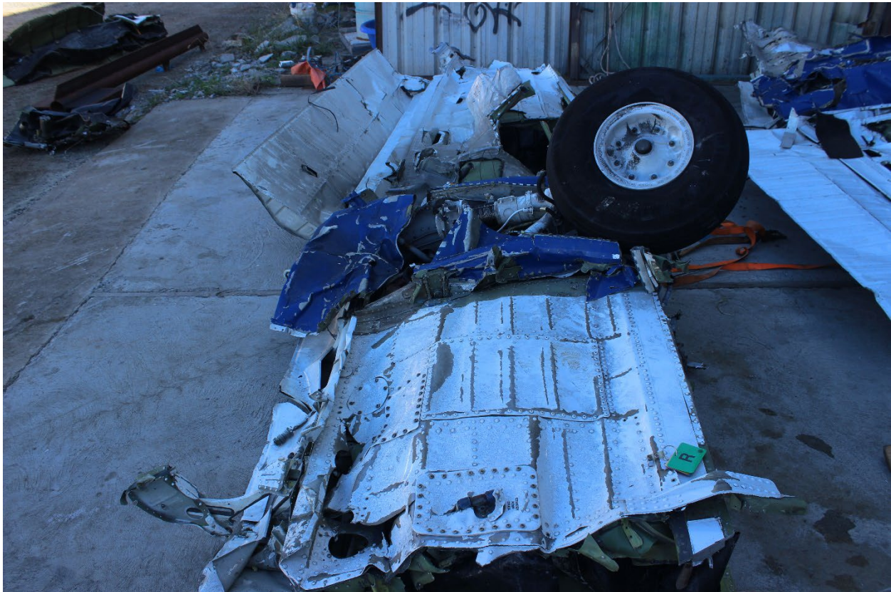
Figure 2 View of the right wing.
