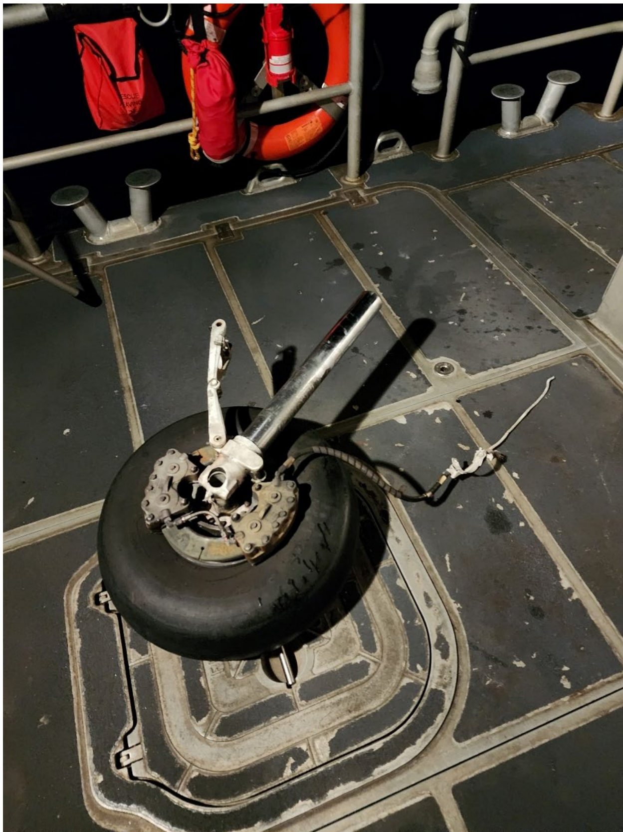
Figure 4 View of left main landing gear recovered by the USCG.
