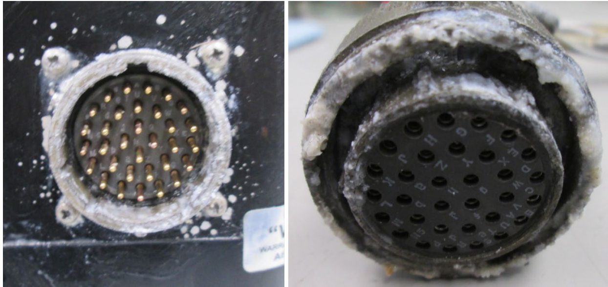
Figure 9. Photo of vertical gyro electrical connector and mating electrical harness connector.
