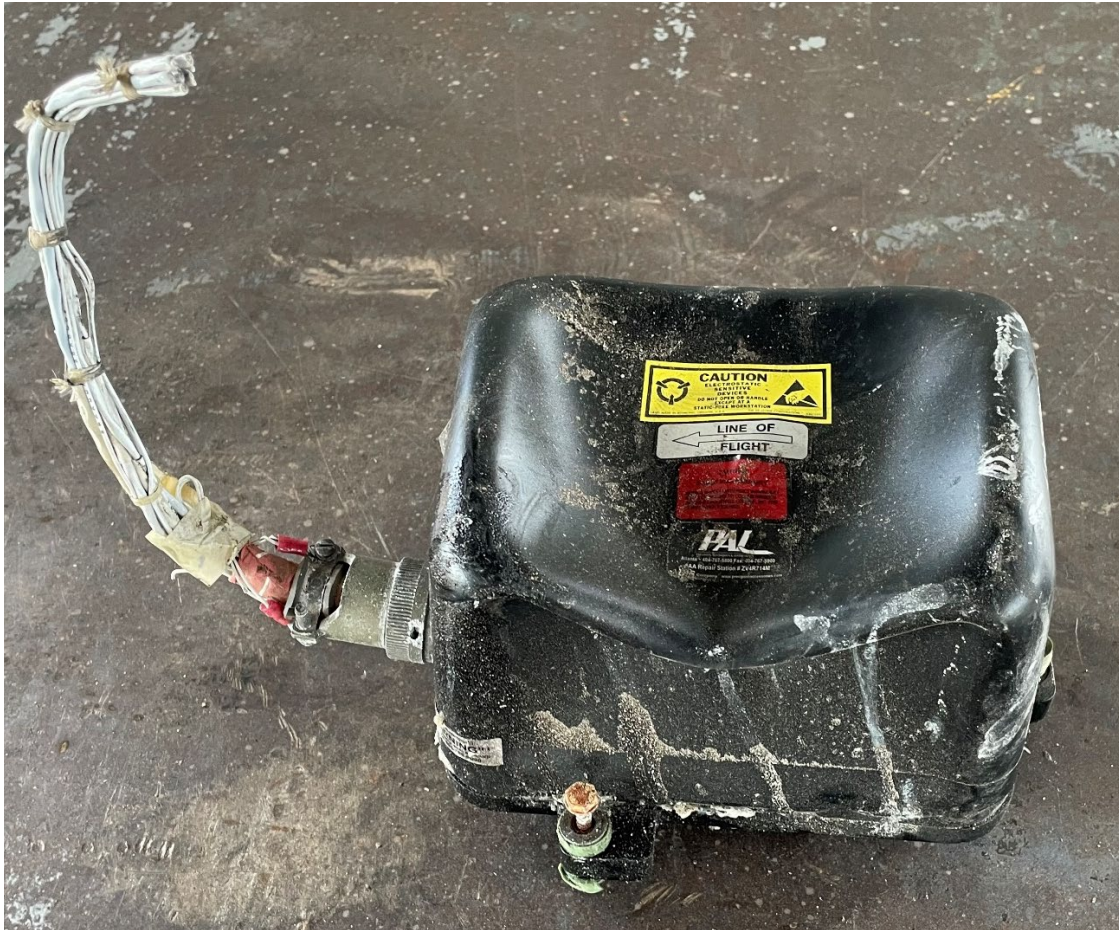
Figure 6. Photo of vertical gyro after removal from wreckage.
