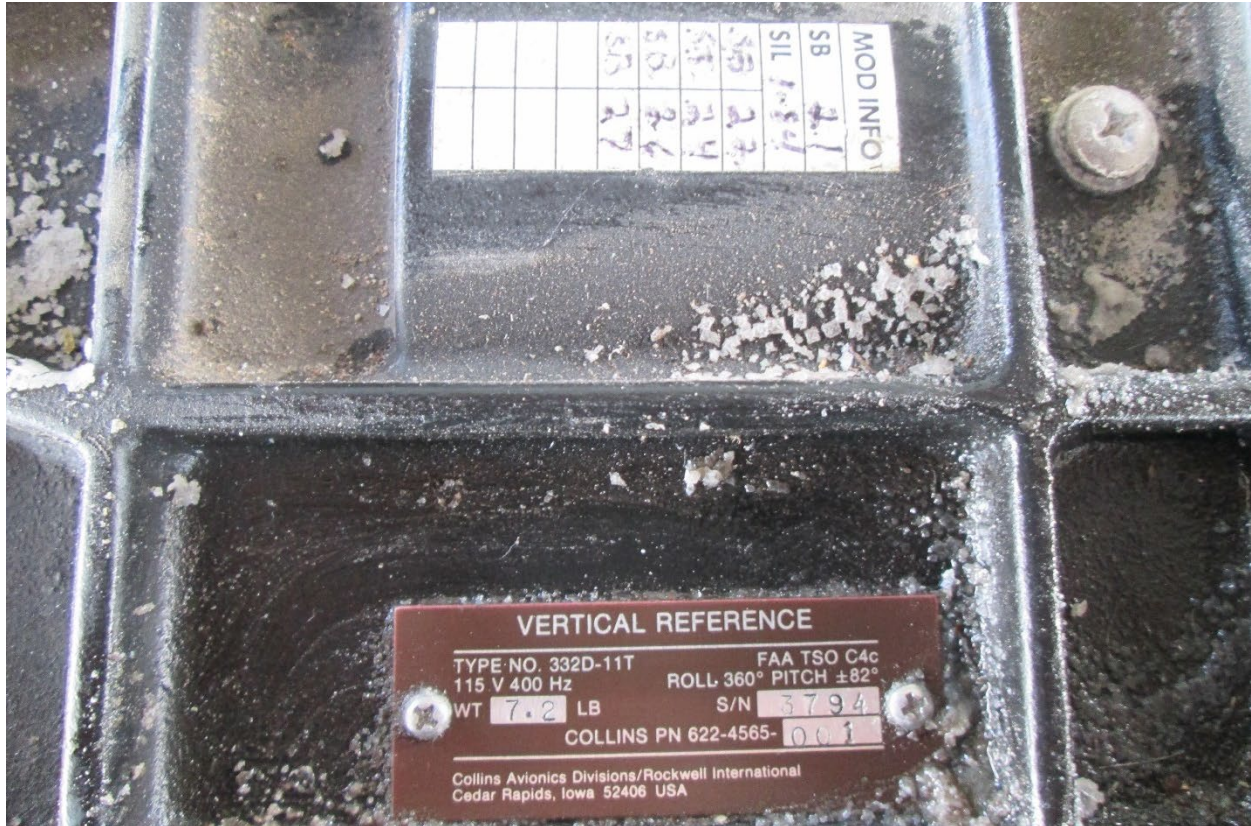
Figure 7. Photo of vertical gyro nameplate.
