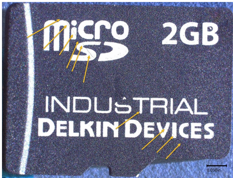
Figure 7. The front the microSD card. The area of the crack is noted with yellow arrows.
