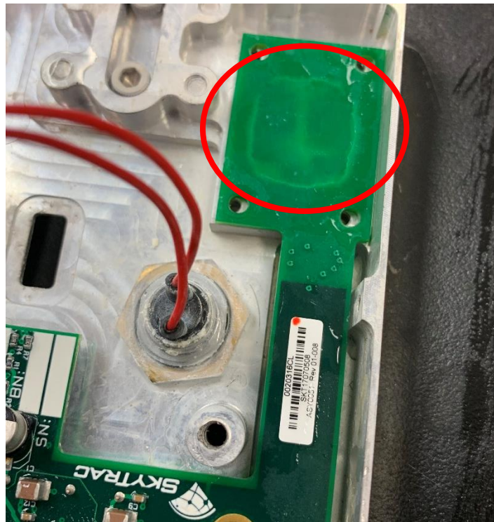
Figure 3. The area of the unit that holds the microSD card with the backing plate removed. Note the area of the concave impression.
