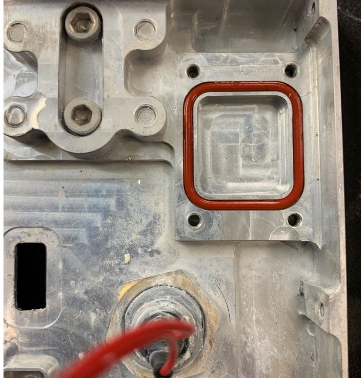
Figure 6. The area of the unit that holds the microSD card with the backing plate removed and the board containing the concave impression/microSD card mount removed. A sealed void space is present.
