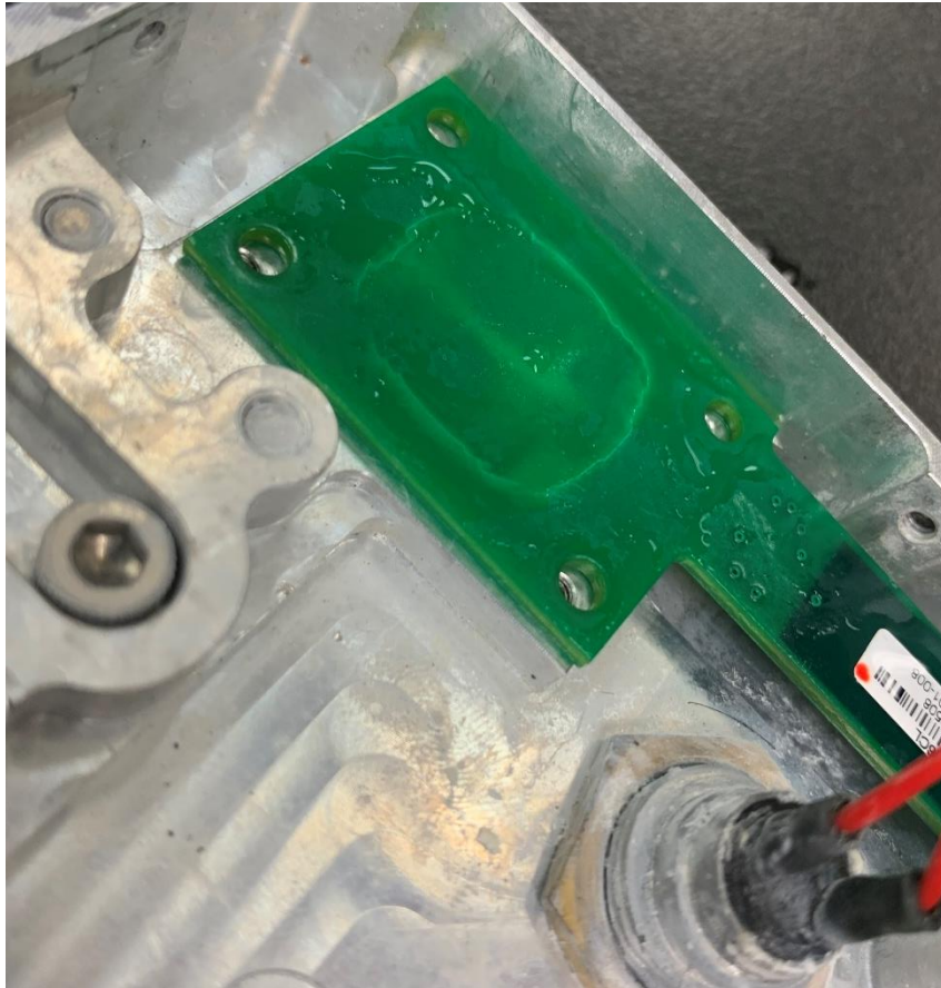
Figure 4. An alternative view of the same area with the concave impression.
