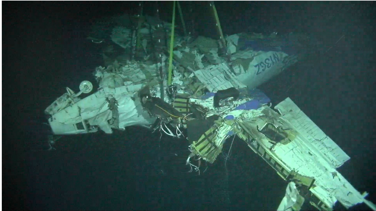
Figure 9. Airplane recovery lift strap orientation (OI photo)
