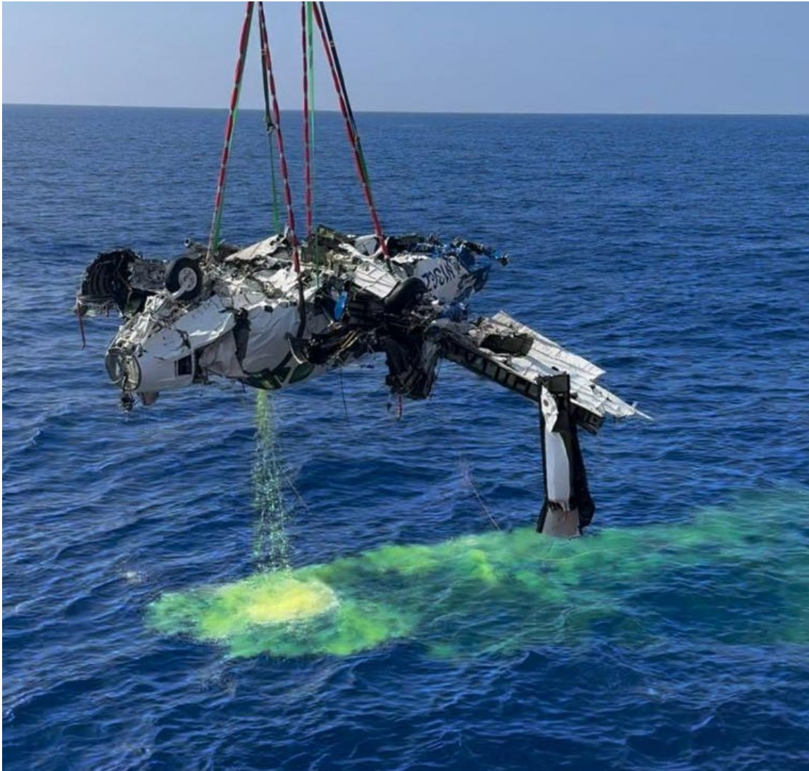
Figure 10. Green dye on water during airplane recovery (OI photo)
