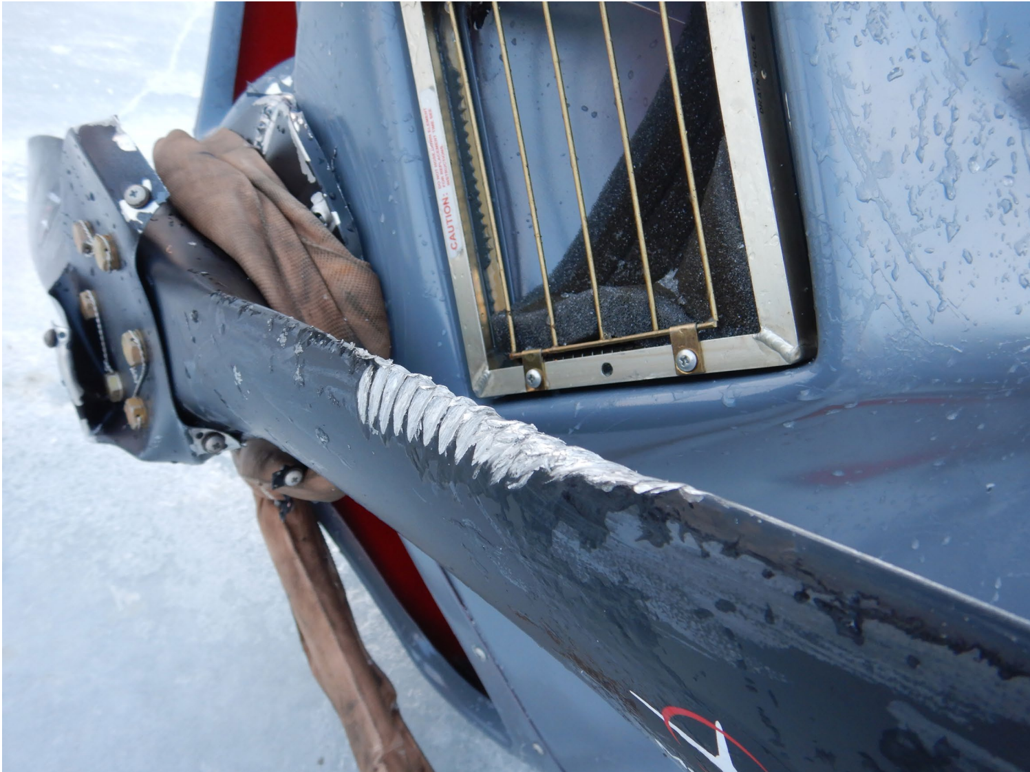
Photograph 2 - View of propeller damage on accident airplane.
