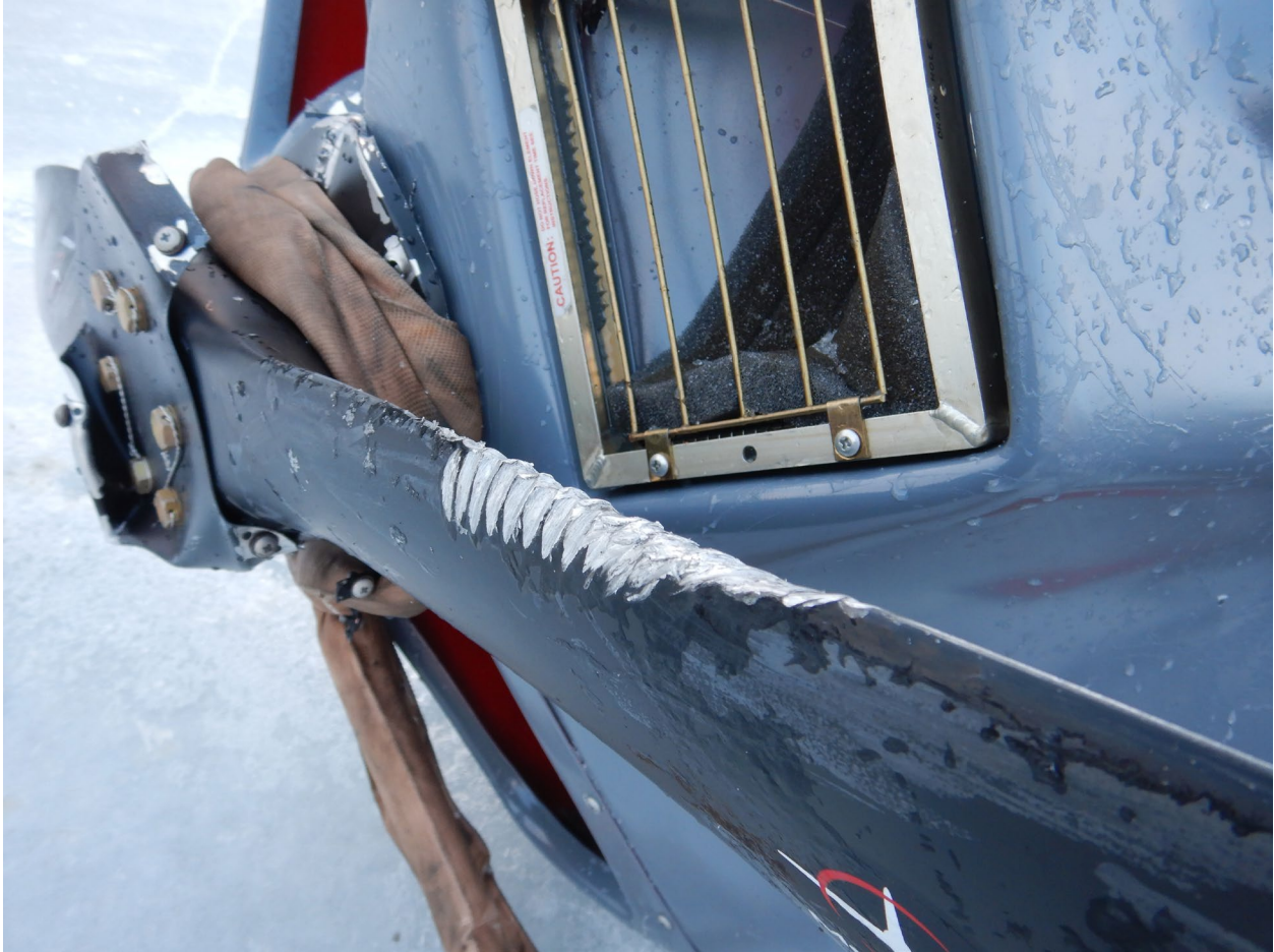
Figure 14 View of damage to the propeller caused by contact with the cable under power.
