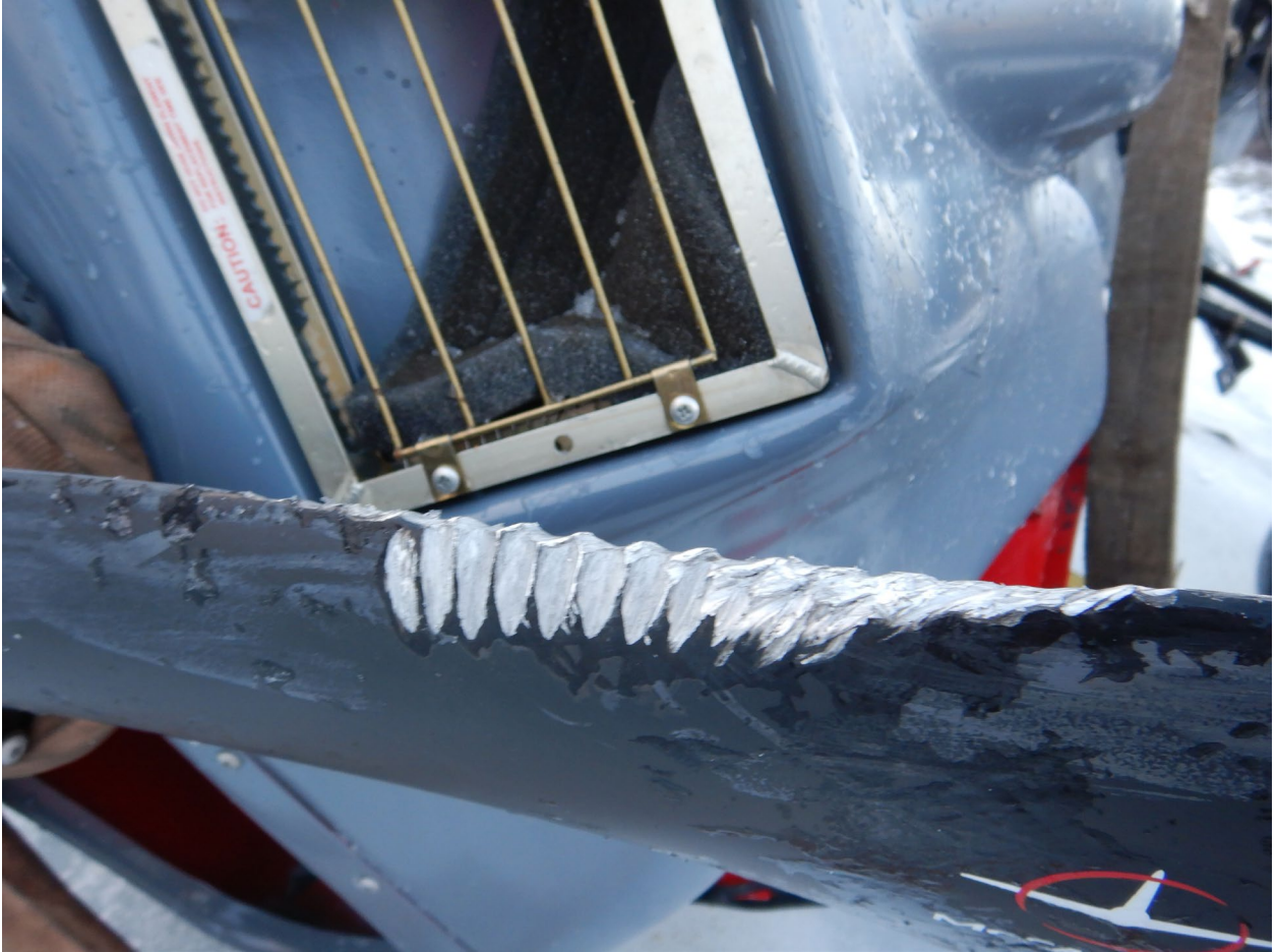
Figure 15 Close up view of the damage to the propeller.
