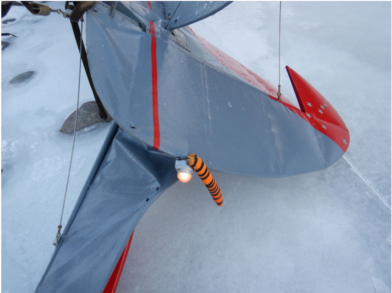
Figure 7 View of left side of the rudder. Battery power was still on.
