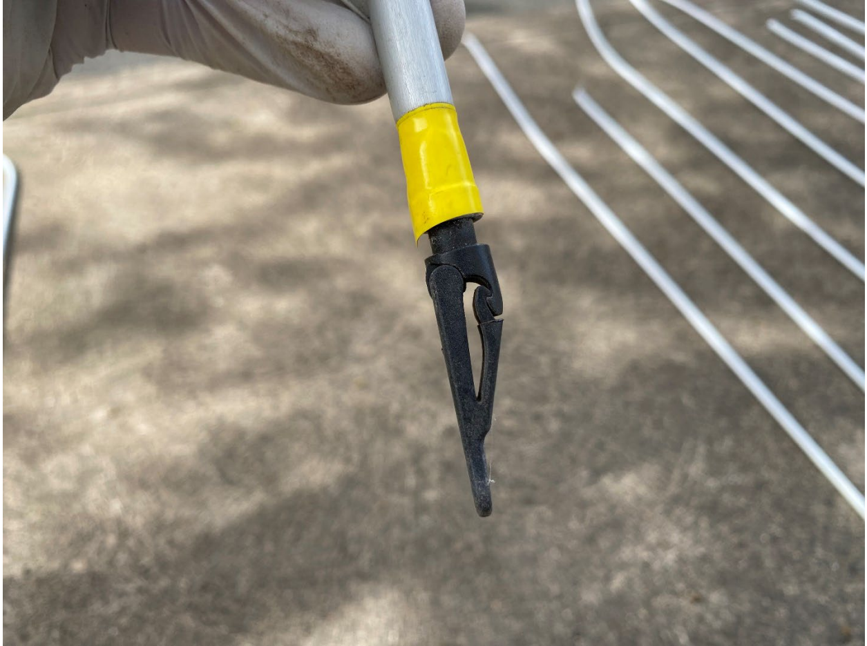
Figure 4 View of one of the remaining hinged batten fittings.
