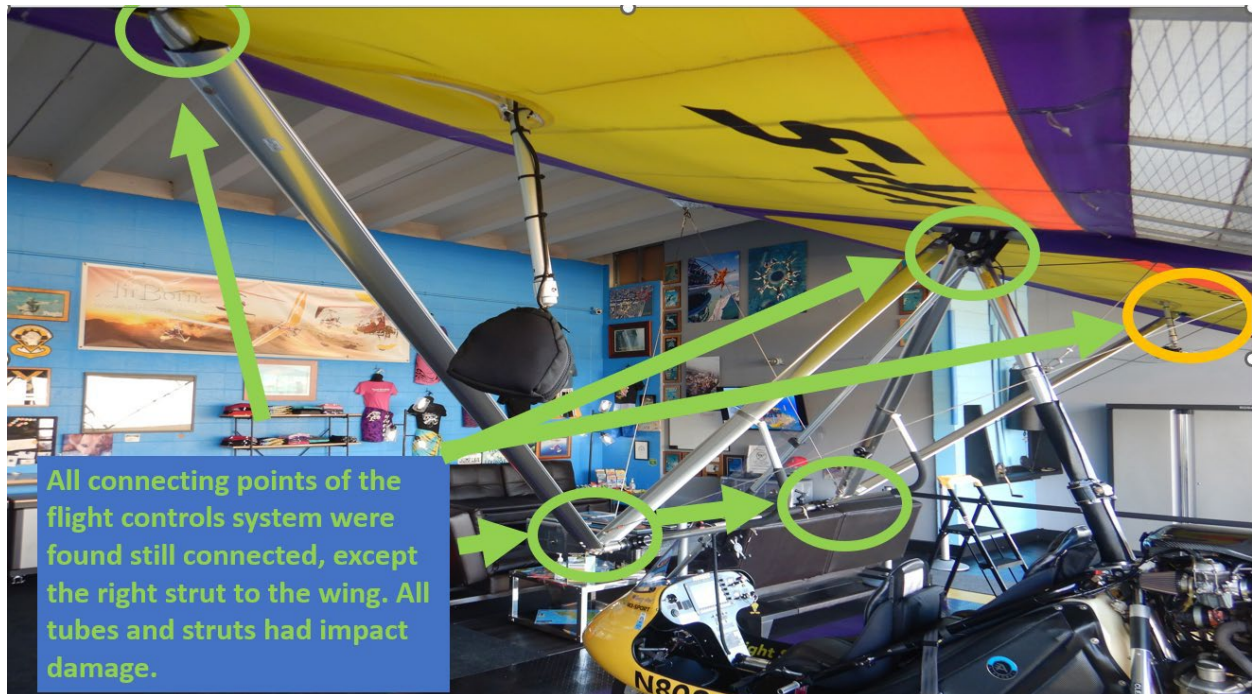
Figure 2 Illustrated exemplar aircraft flight control connecting points
