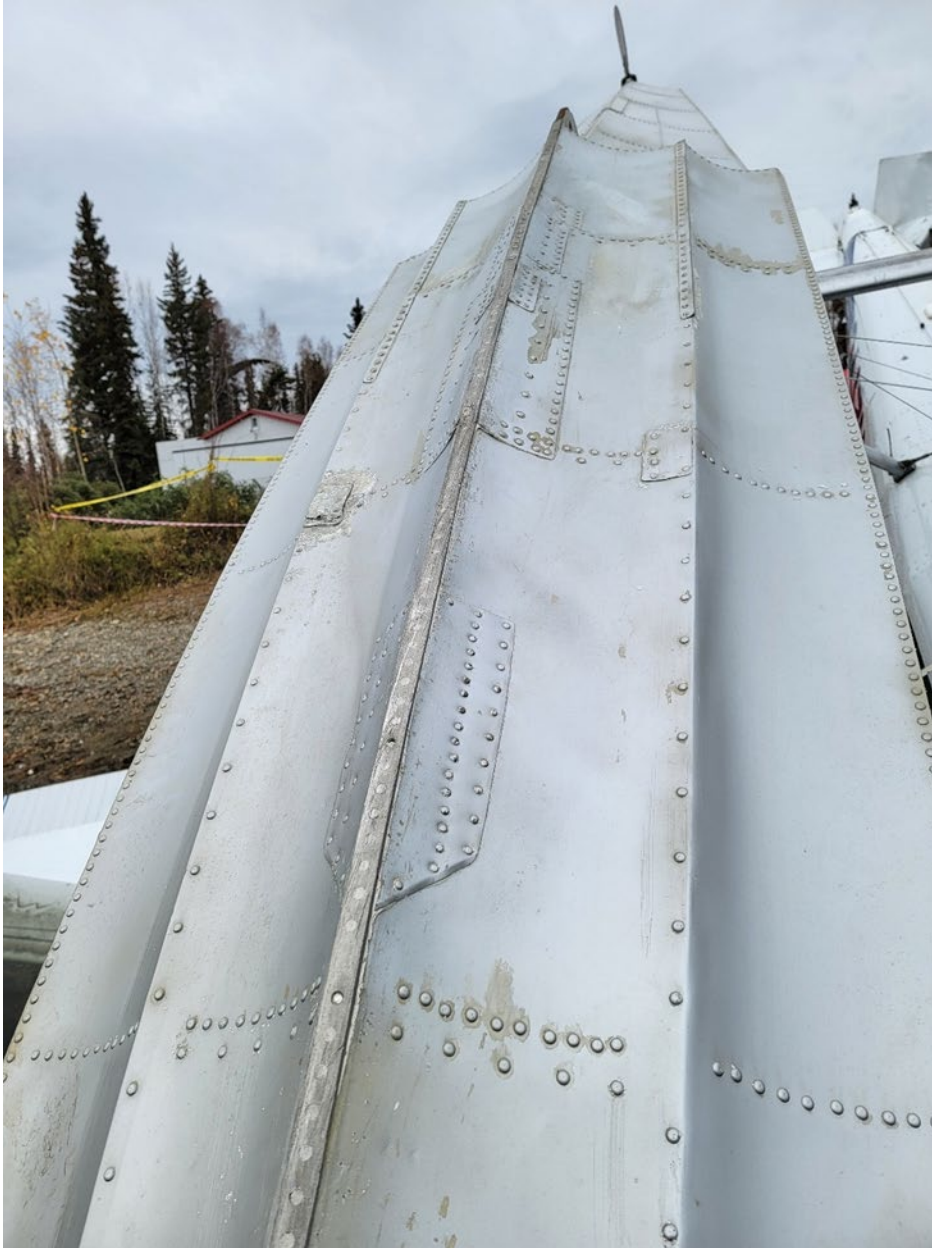
Figure 4 Left under side of float. Showing wear on the keel.
