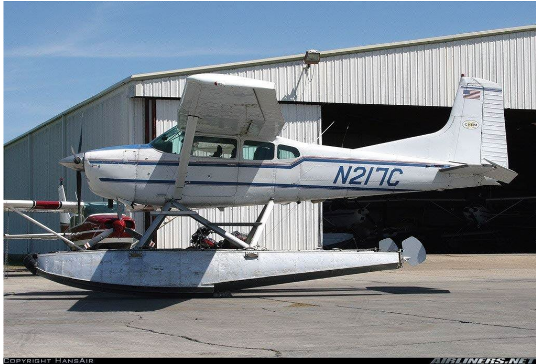
Figure 1 Undated photo of N217C with modified front float bumpers
