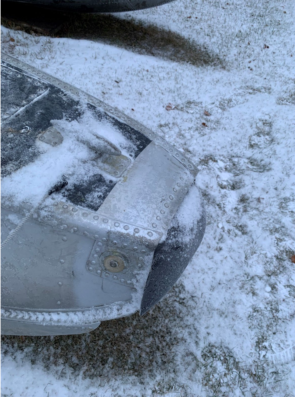
Figure 3 New bumpers installed by owner
