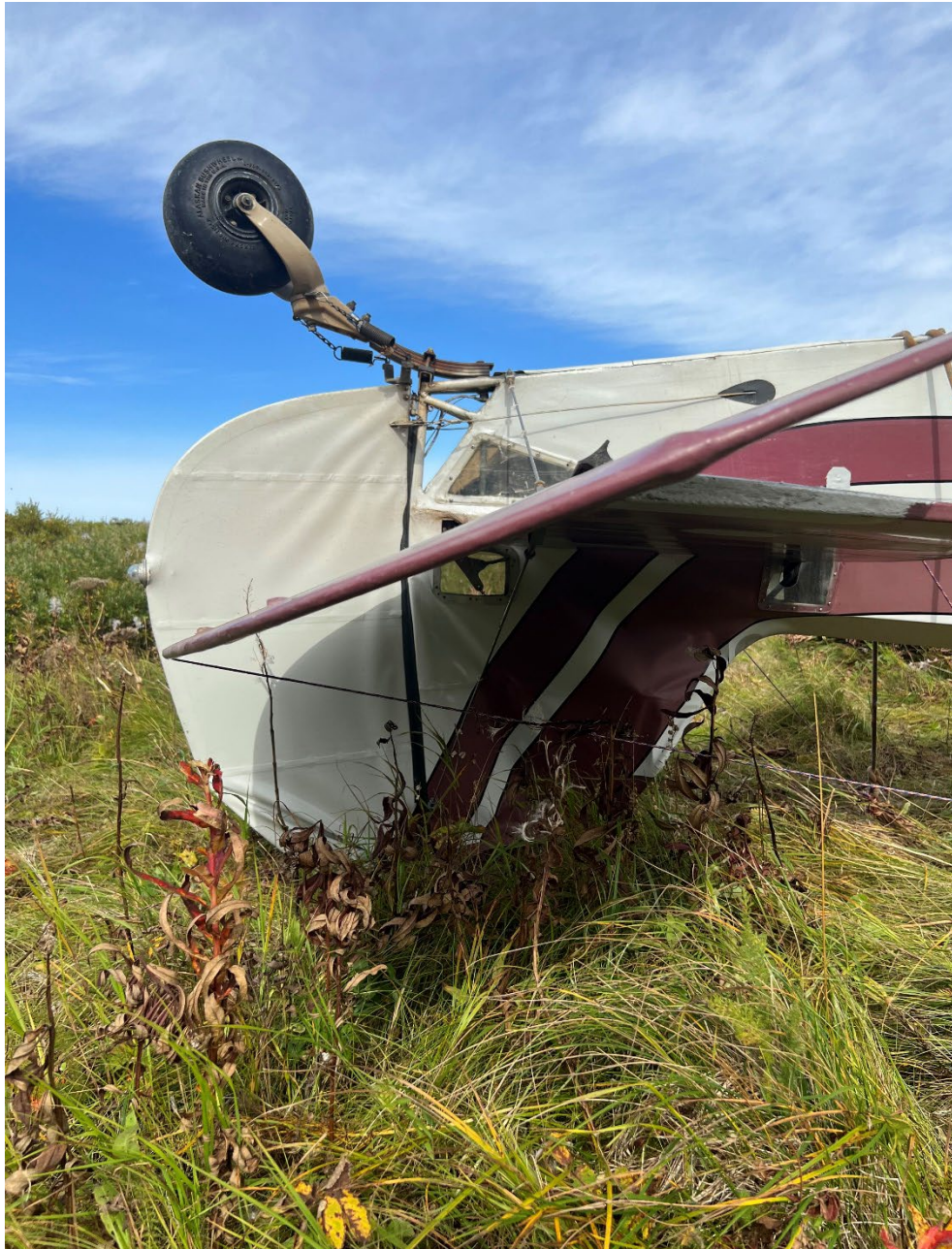
Photo 3 – View of Rudder and Vertical Stabilizer Damage. (Courtesy of Pilot)
