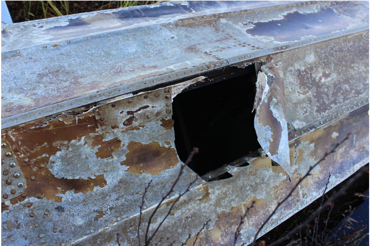
Figure 4 View of the partially separated section of the right float.
