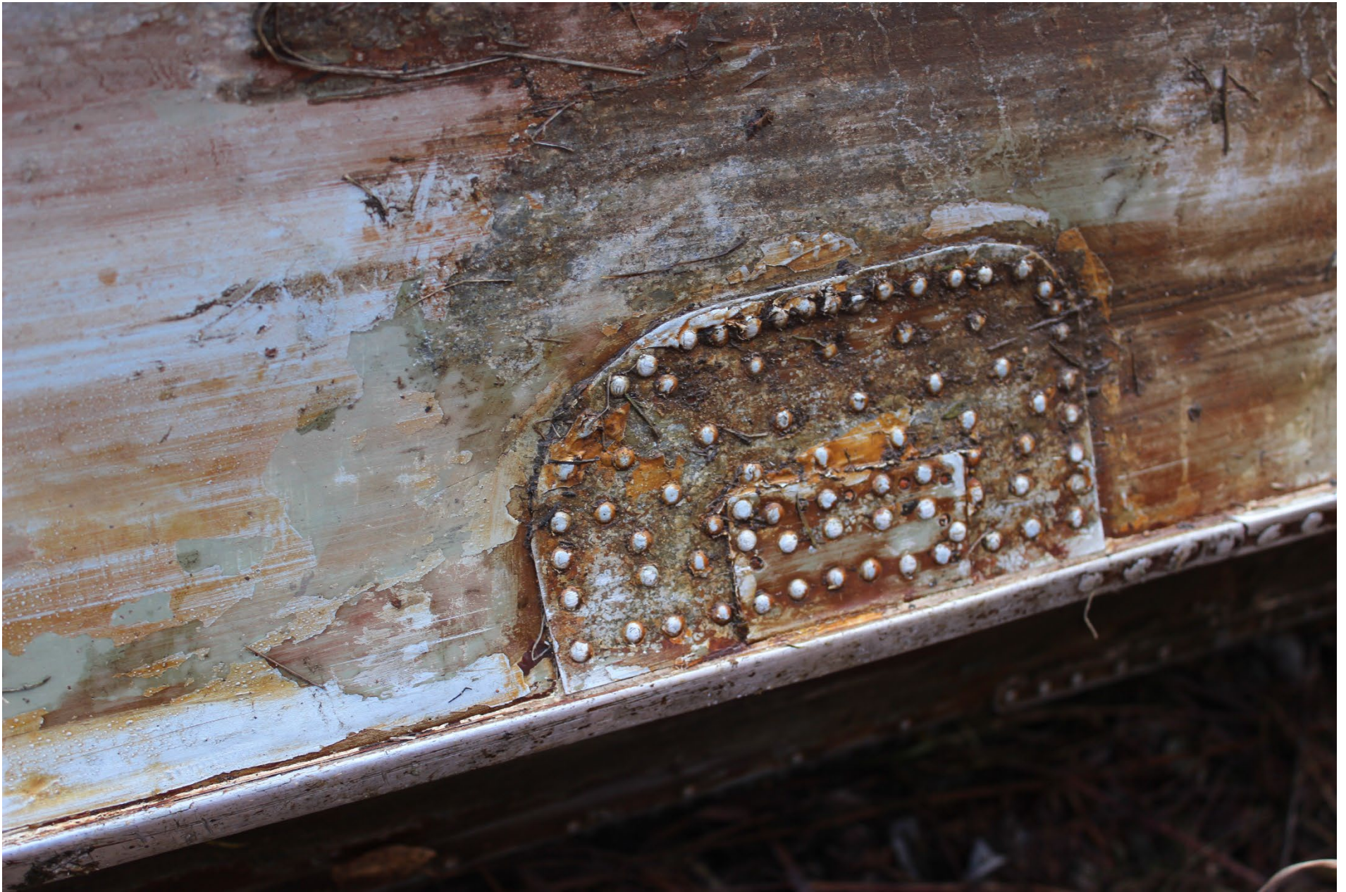
Photo 7 - View of multiple patches on the left float.
