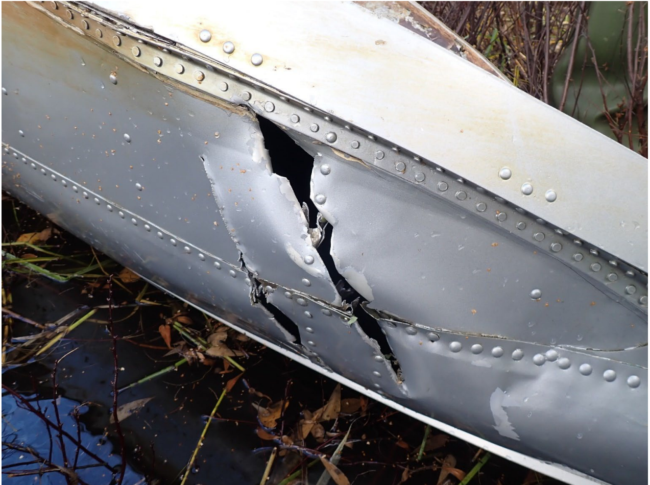
Propeller strike damage, ASI-22-CI-070
