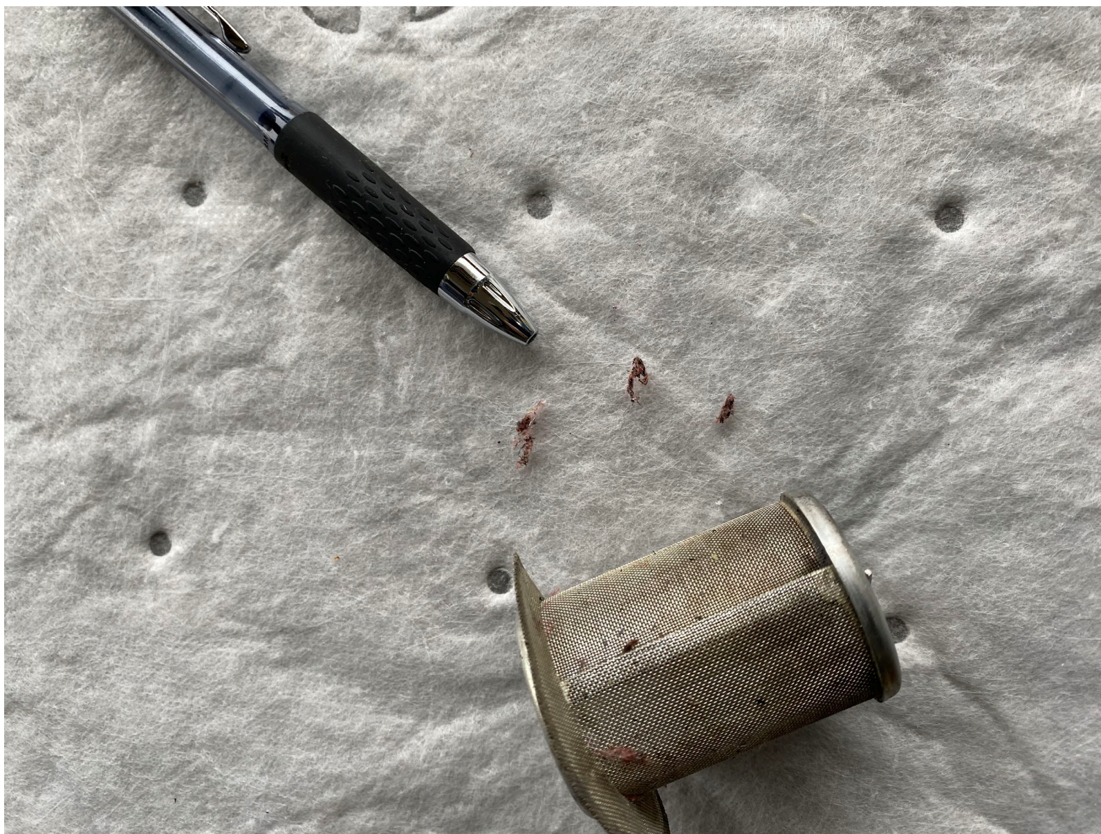
Photograph 8 - Fuel screen debris (Courtesy of FAA)
