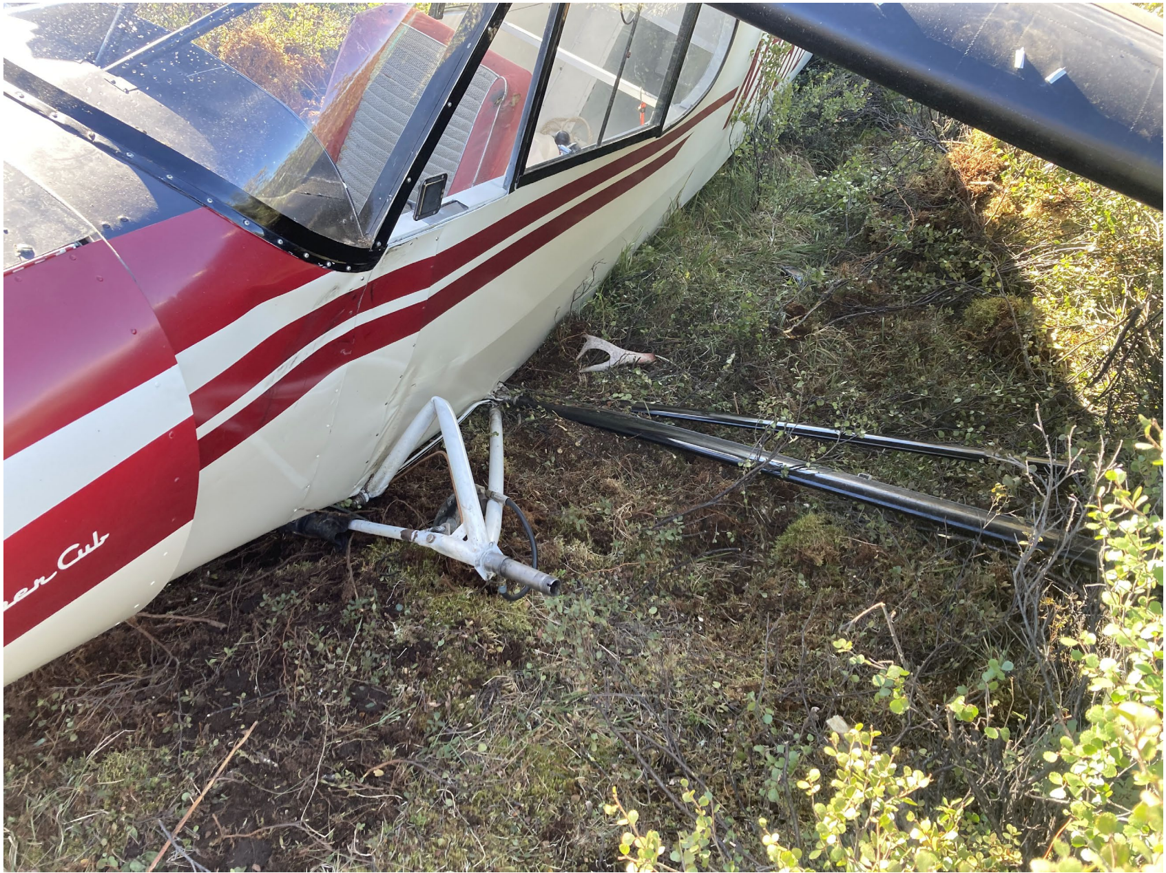
Photo 2 – Damaged left wing strut (Courtesy of Alaska Wildlife Trooper)
