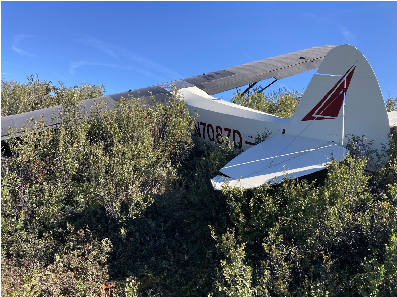
Photo 3 – Damaged left elevator (Courtesy of Alaska Wildlife Trooper)
