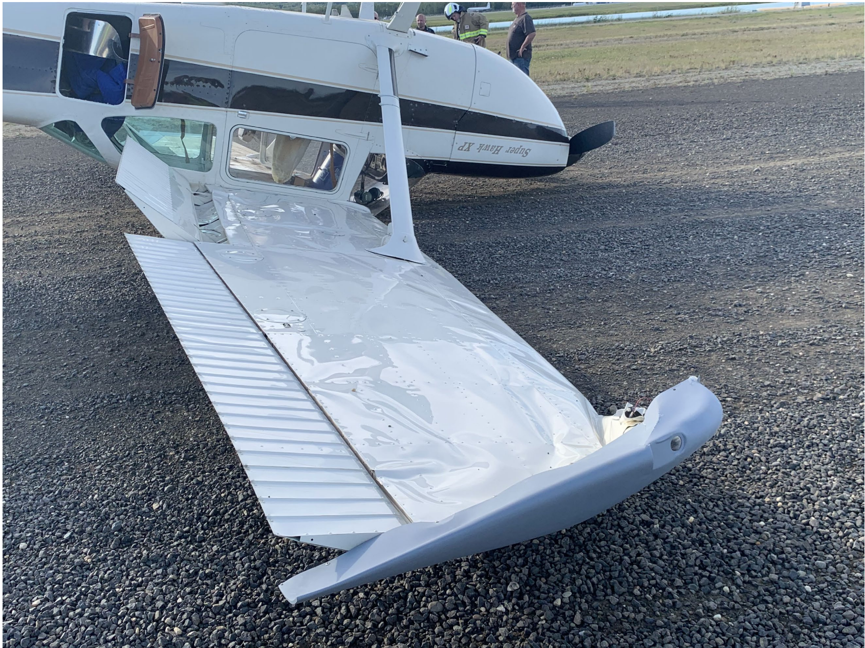
Photo 2 – Left wing damage (courtesy of FAI airport operations)
