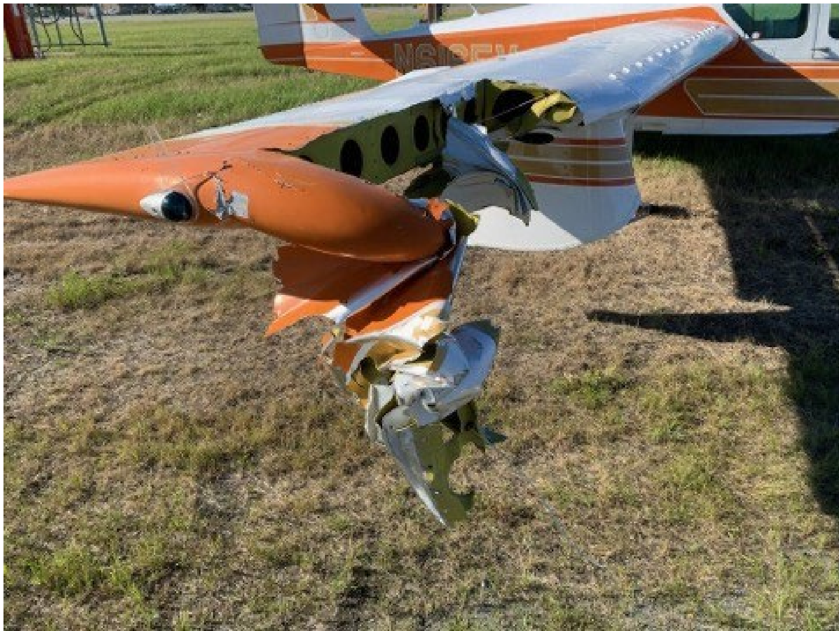
Photo 2 – Accident airplane's substantially damage left wing.
