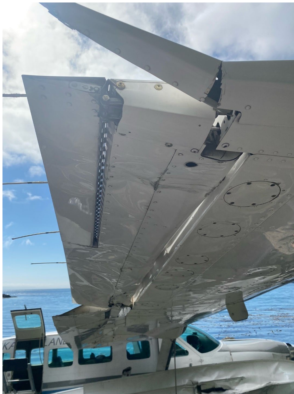
Photo 2 – The accident airplane’s substantially damage right wing and aileron. Photo provided by Alaska Seaplanes.
