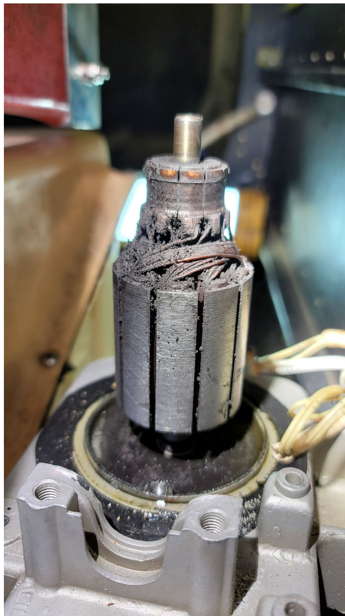
Photo 5 – Accident airplane’s landing gear hydraulic power supply’s reversible electric-motor’s rotor. Photo provided by FAA.
