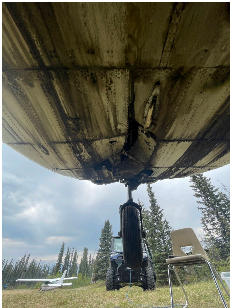
Photo 2 - Photo of accident airplane which depicts substantial damage to lower fuselage/belly. (Photo provided by operator via FAA)
