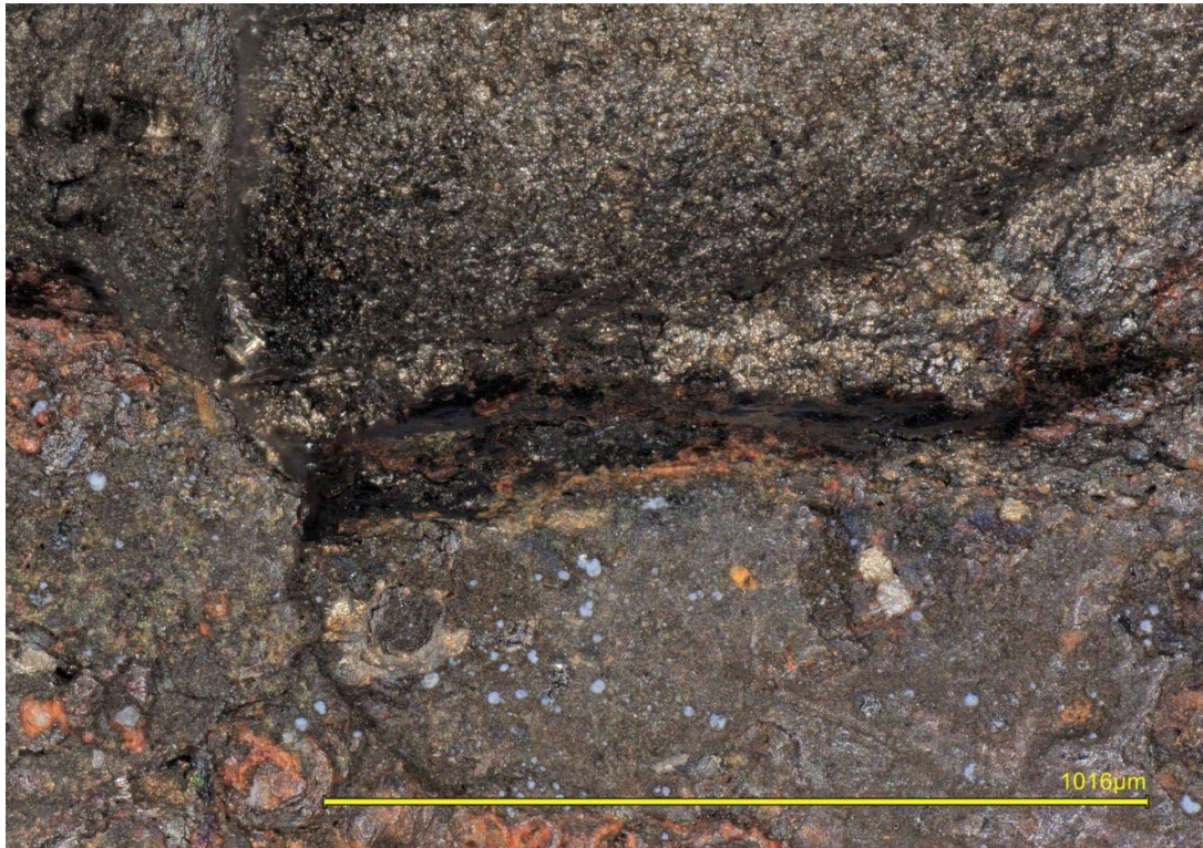
Figure 19. Closer view of the right initiation side from the surface edge in Figure 18.
