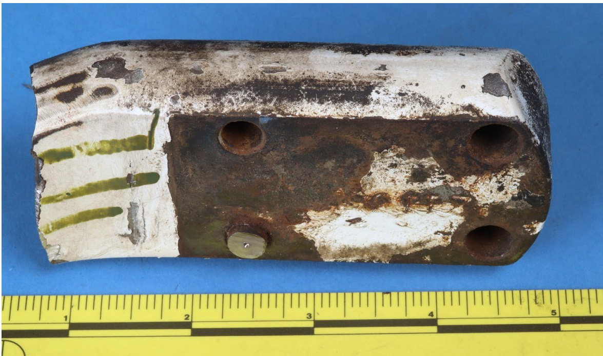
Figure 2. Angled view of the leg fragment opposite that of Figure 1, showing a bend towards the fracture surface.
