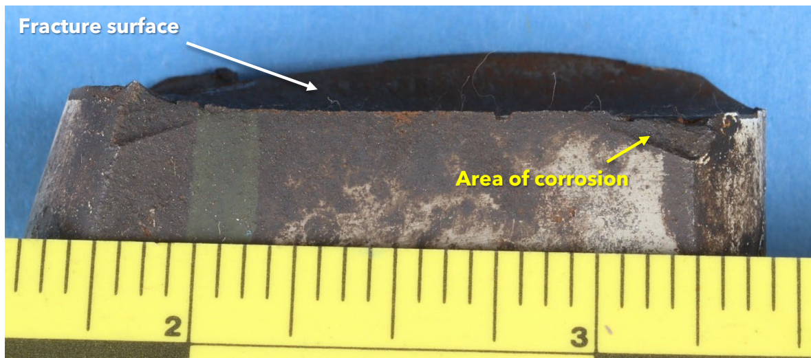
Figure 7. View from underneath of the leg, showing the area of corrosion and the fracture surface.
