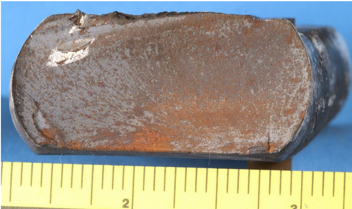
Figure 4. View of the leg fragment fracture surface, as received.
