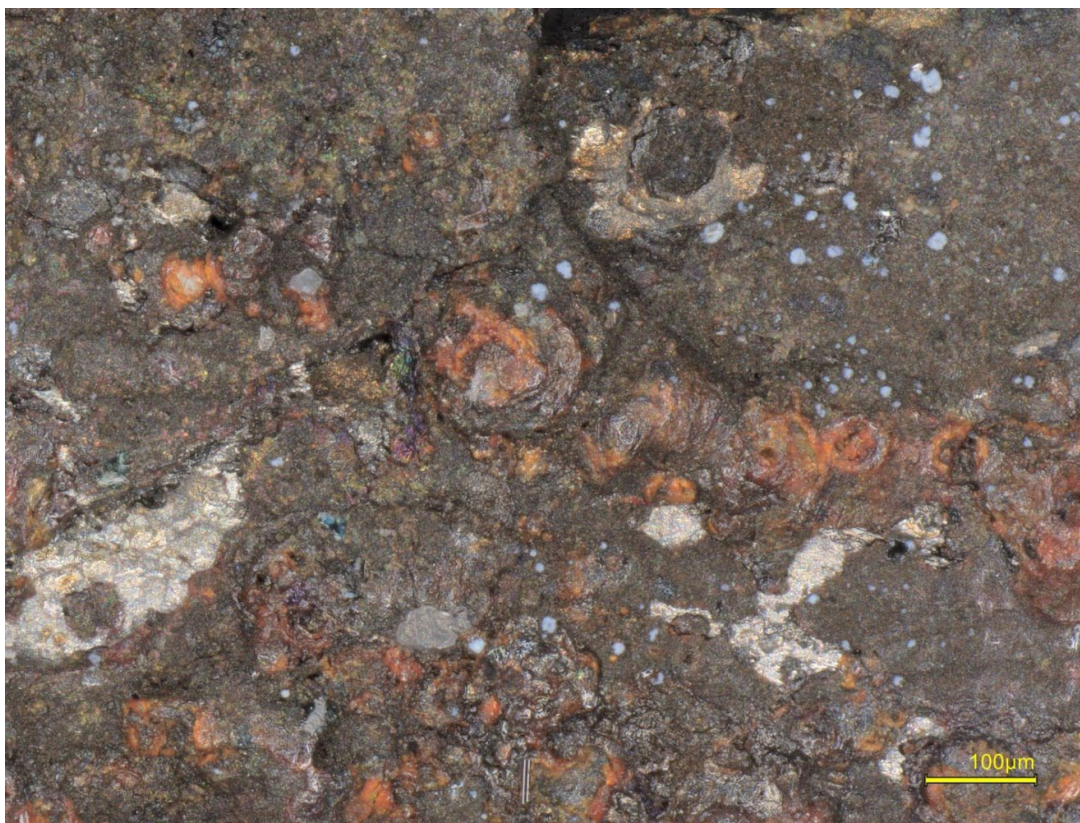
Figure 21. Pitting corrosion and corrosion compounds on the underside of the leg remnant adjacent to the fatigue crack initiation sites.
