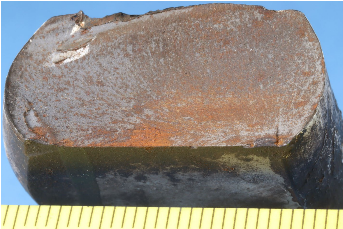
Figure 5. Angled view of the fracture surface edge of the leg fragment, showing the fracture initiation region in the lower right.
