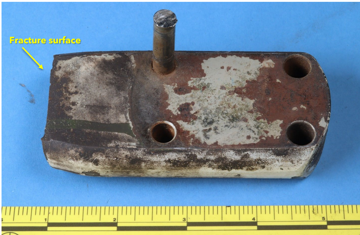
Figure 1. View of the main landing gear leg fragment, as received.
