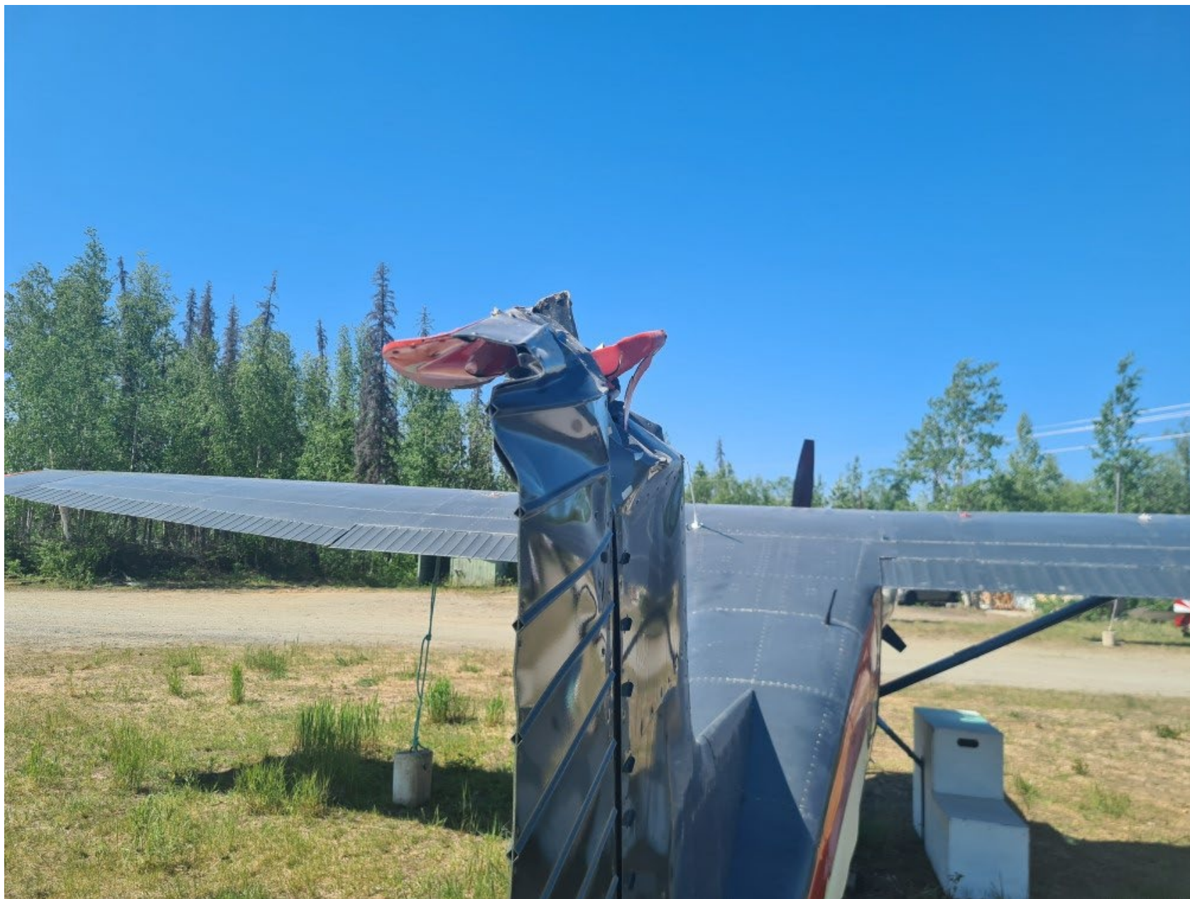
Photo 2 – Accident airplane’s substantially damaged rudder and vertical stabilizer.
