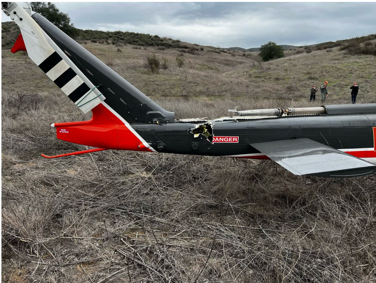
Photo 2 – Right aft view of tail boom, of accident helicopter at accident site. Photo provided by Operator (Heliqwest)
