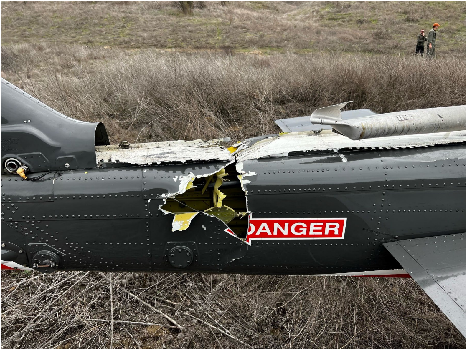
Photo 3 – Aft right-side view of tail boom damage on accident helicopter at accident site. Photo provided by Operator (Heliqwest).
