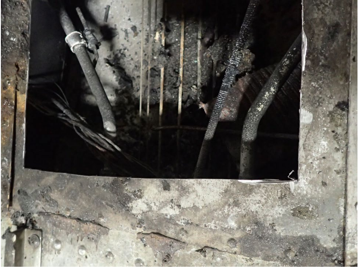
Figure 7 Overhead view of ignition point in fuselage.
