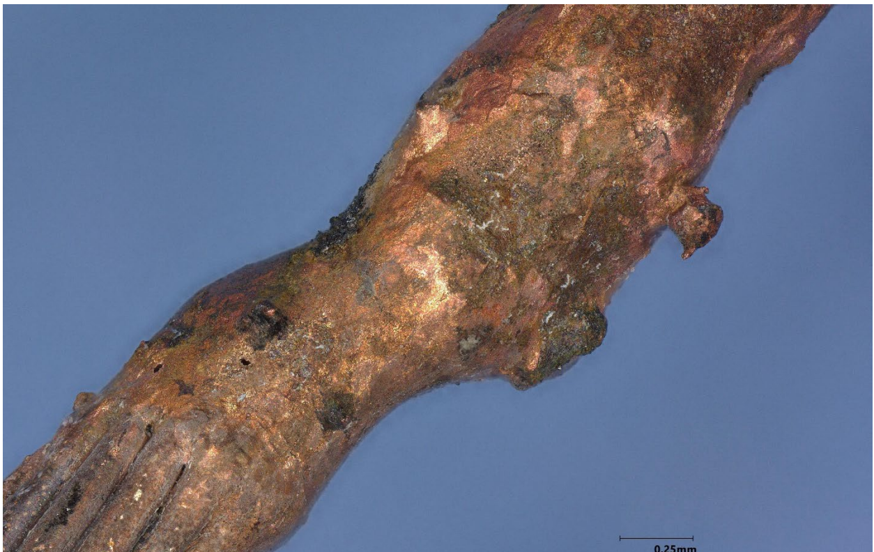
Figure 8. Closeup of welded area on conductor in Figure 7.
