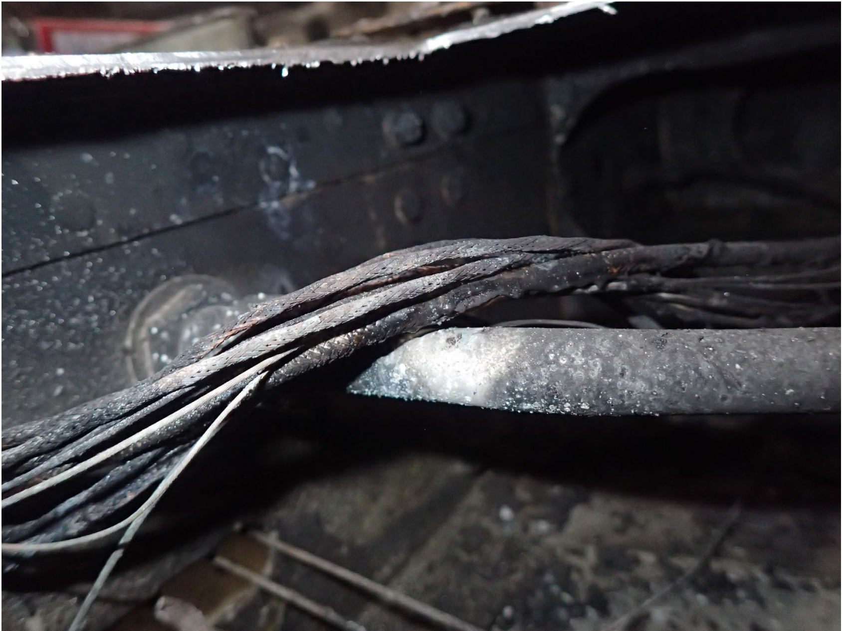
Photo 3 – View of wire bundle over aft left tank fuel line in accident airplane. Photo provided by the NTSB.
