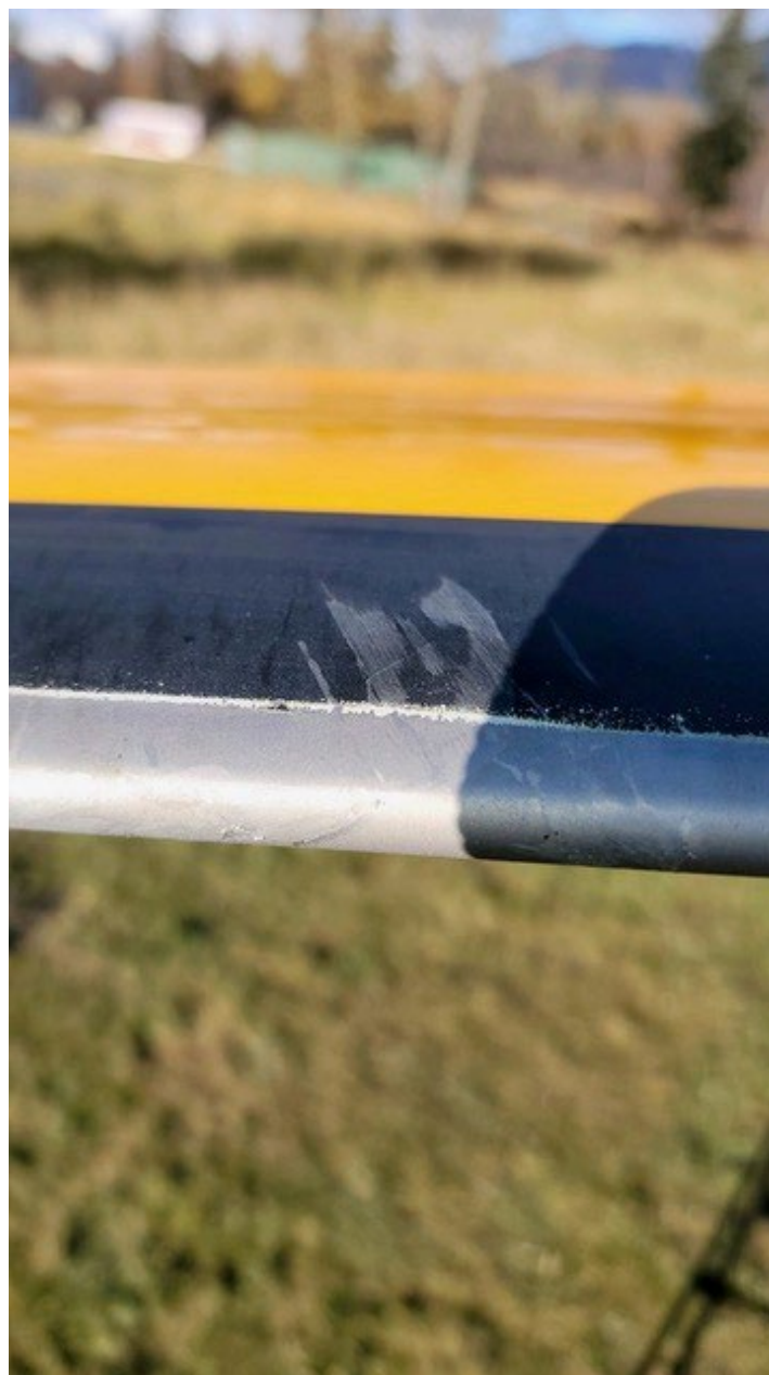
Photo 2 – Accident helicopter's substantially damaged main rotor blade.
