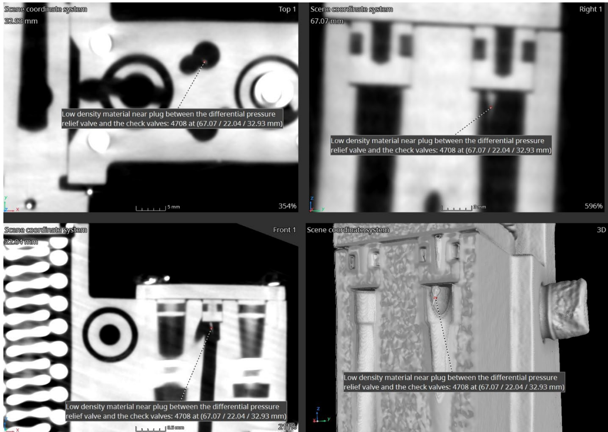
Figure 144. Left lateral actuator - irreversible valve - low density material near plug between the differential pressure relief valve and the check valves. (450 kV)
