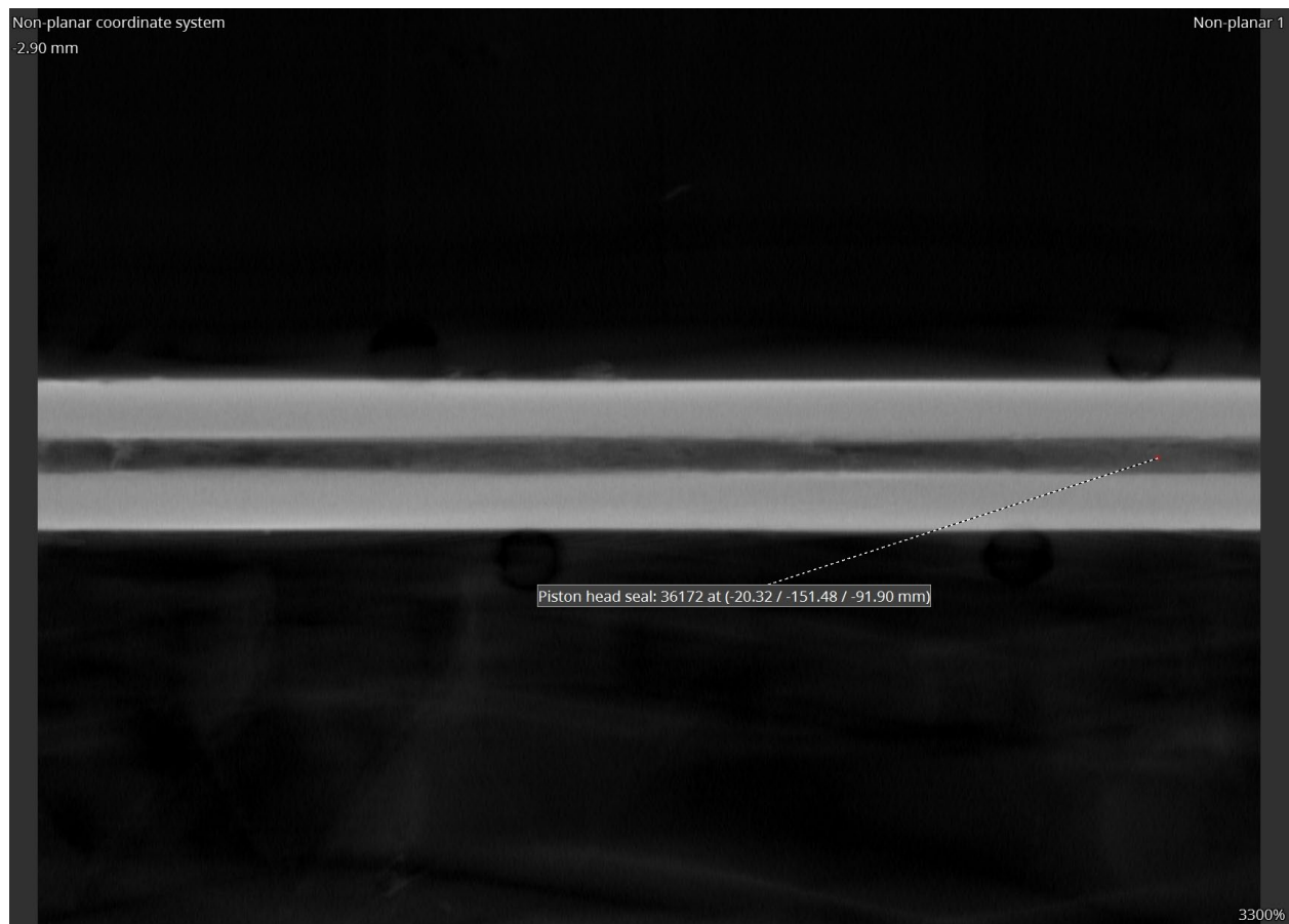
Figure 108. Left lateral actuator - cylinder assembly - piston head seal unrolled.
