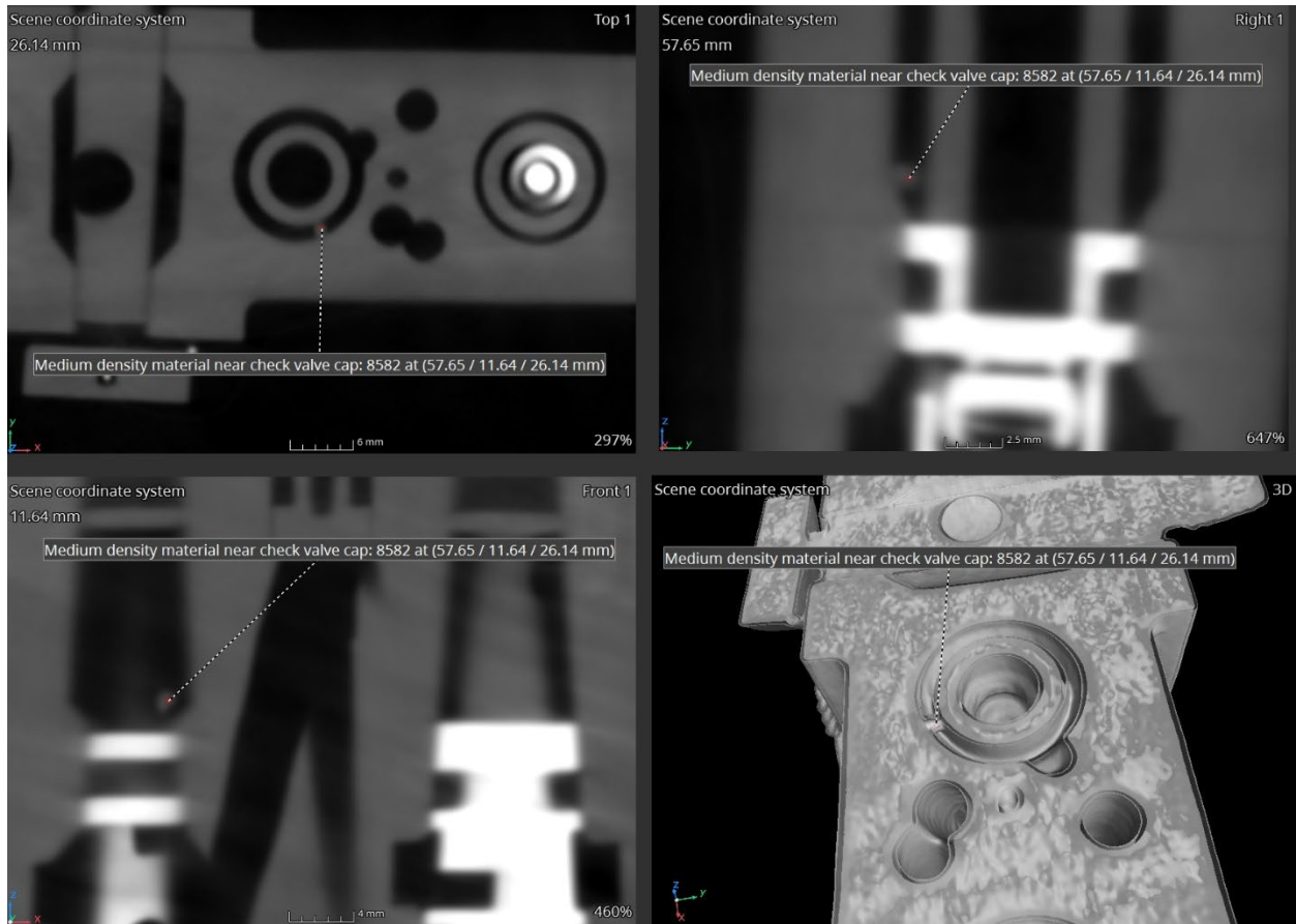
Figure 138. Left lateral actuator - irreversible valve - check valve B - medium density material. (450 kV)
