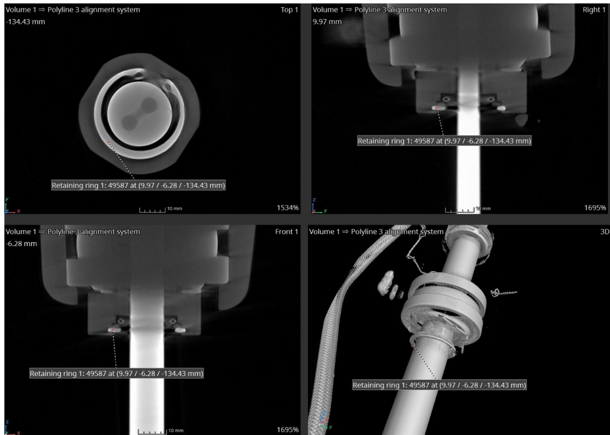
Figure 85. Right lateral actuator - cylinder assembly - retaining ring 1. (225 kV)
