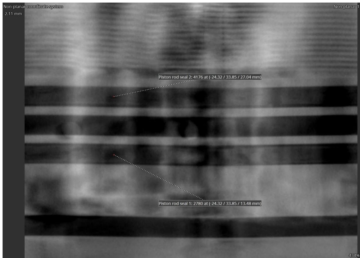
Figure 79. Right lateral actuator - cylinder assembly - piston rod seals 1 and 2 unrolled. (450 kV)
