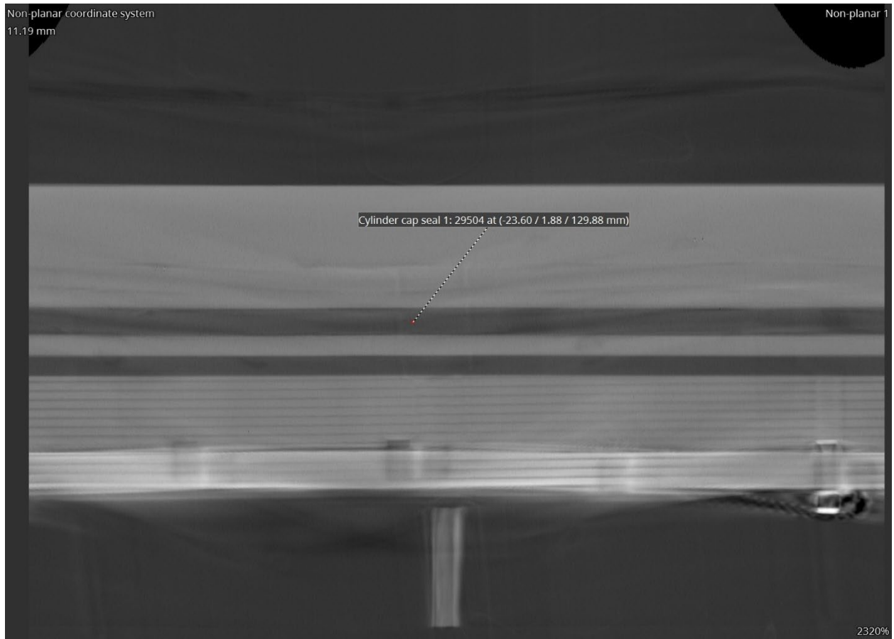
Figure 48. Collective actuator - cylinder assembly - cylinder cap seal 1 unrolled. (225 kV)
