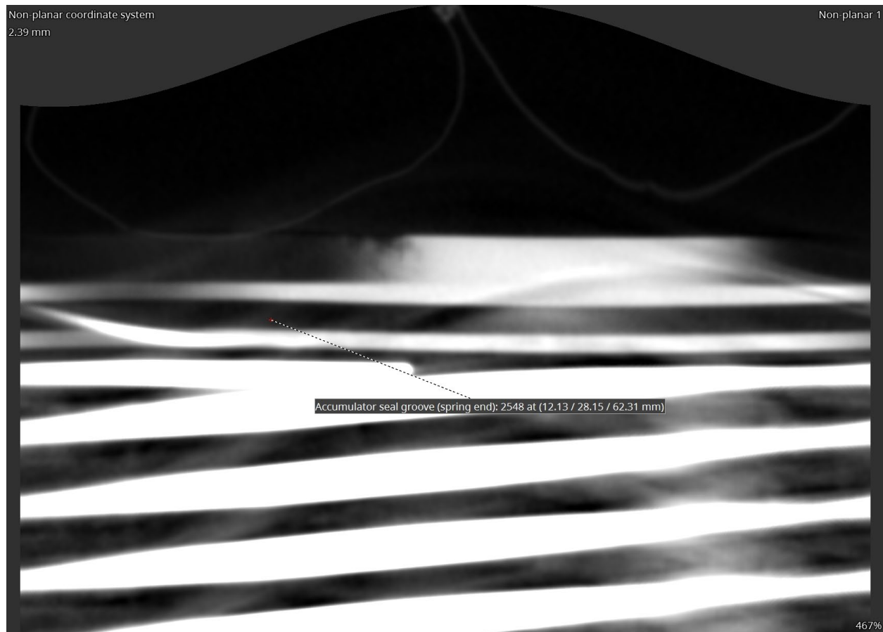
Figure 154. Left lateral actuator - irreversible valve - accumulator seal groove unrolled at spring end. (450 kV)
