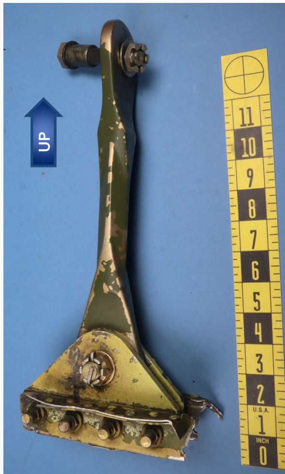
Figure 1. Overall view of the submitted lift link assembly with attached fuselage beam structure piece (left) and view of fractures on the lower side of the submitted beam structure piece (below).
