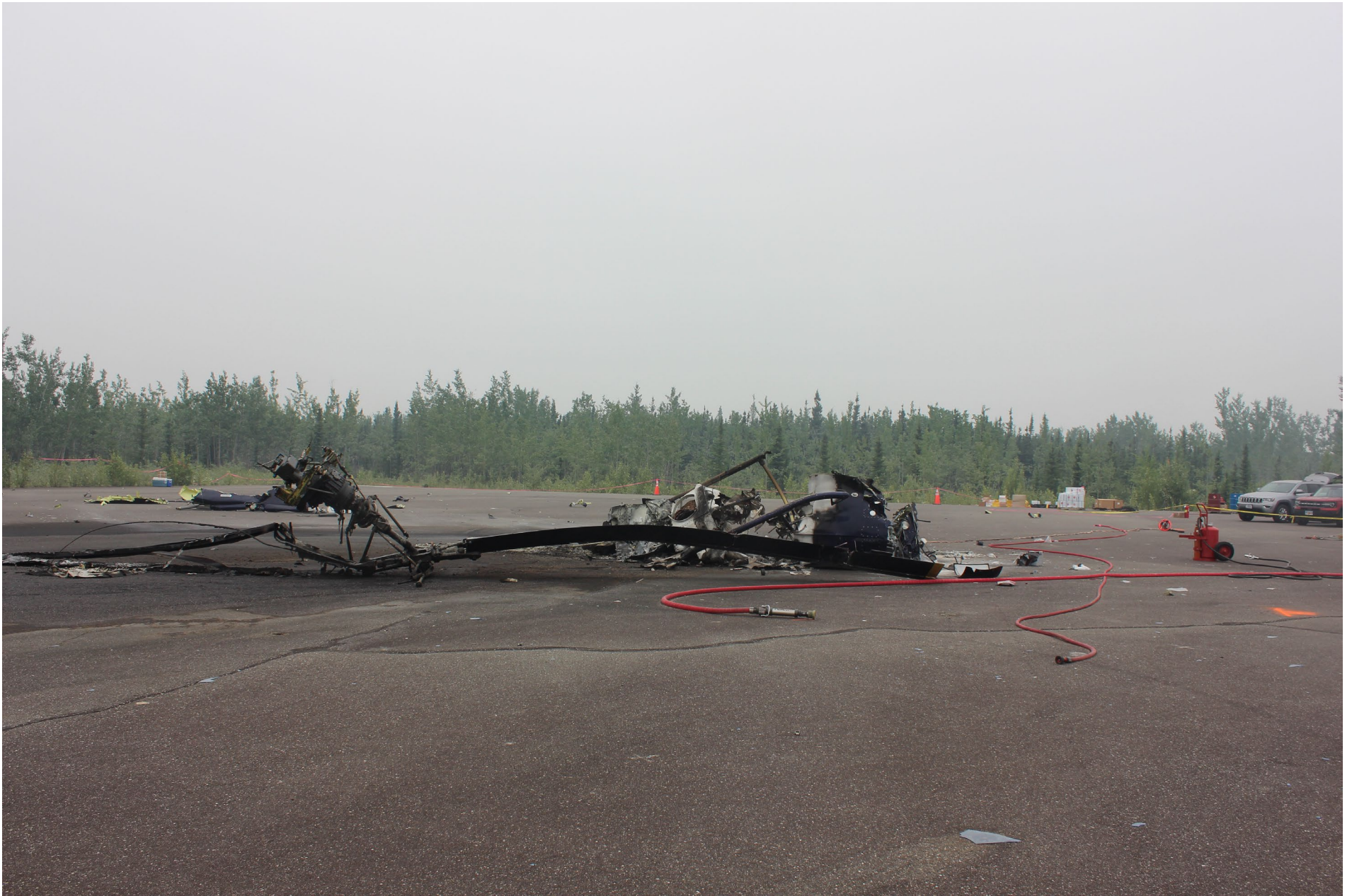
Photo 3 – The accident helicopter’s separated transmission and rotor head with the blades still attached.
