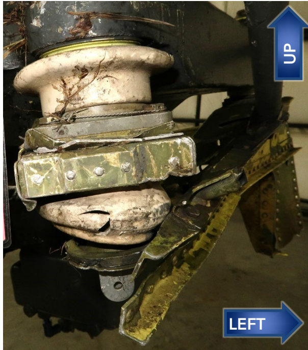
Figure 2. Close views of the fractured pylon support legs at the forward left (left image) and forward right (right image) main transmission attachment locations.
