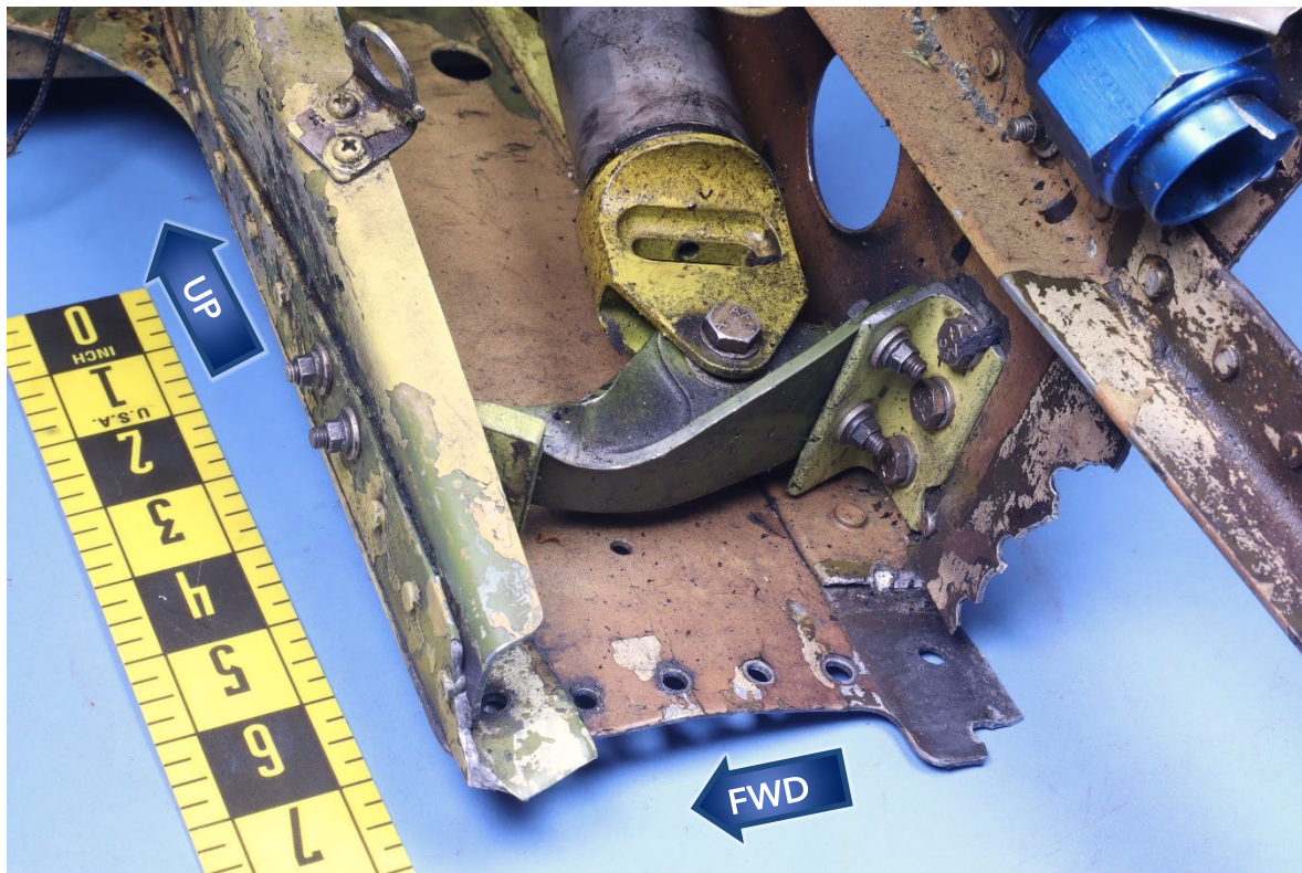
Figure 9. Lower ends of the aft left (upper image) and aft right (lower image) pylon support pieces after disassembling the isolation mounts and upper portions of the friction dampers.
