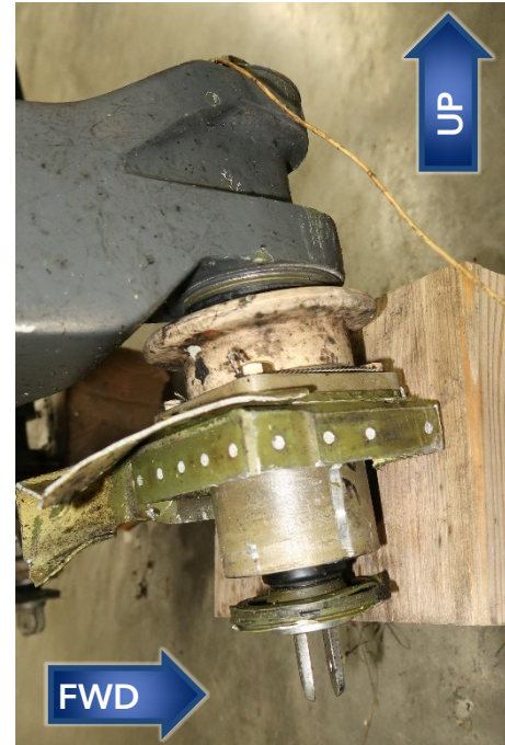
Figure 2. Close views of the fractured pylon support legs at the forward left (left image) and forward right (right image) main transmission attachment locations.
