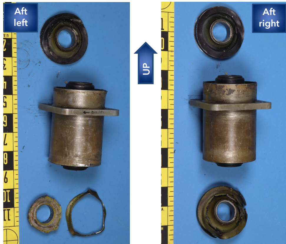
Figure 11. Aft left and aft right isolation mounts and bushings after disassembly from the isolation mount bolts.
