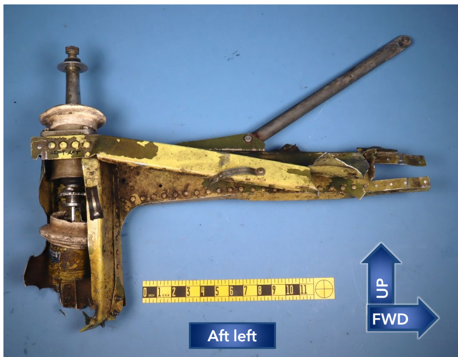
Figure 8. Aft pylon pieces after disassembling the main transmission case from the aft isolation dampers.
