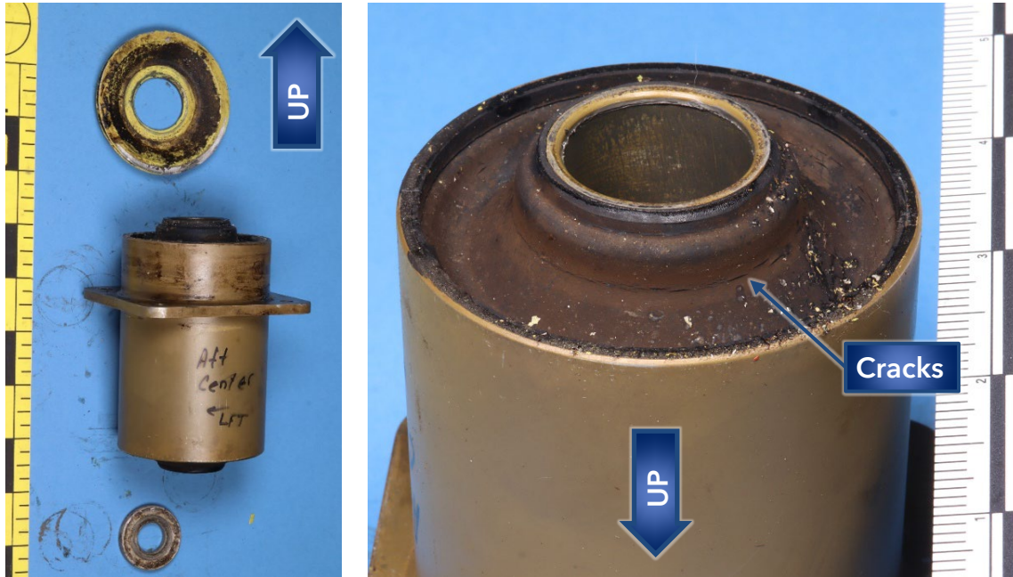
Figure 14. Aft side of the aft center isolation mount, bushing, and washer (left image) and lower end (right image) after disassembly from the pylon aft beam.
