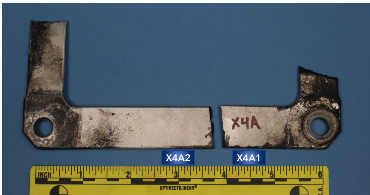
Figure 1. Overall view of the submitted KAflex coupling pieces as received.
