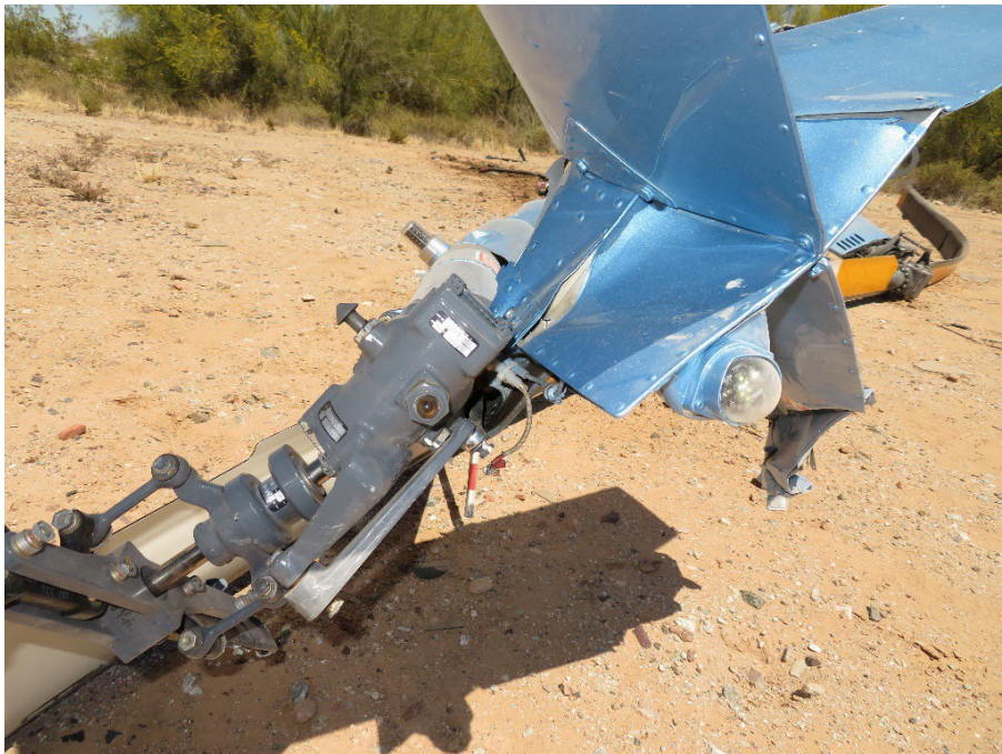
Photo of tail rotor gearbox, tail rotor hub linkages, looking south (NTSB Photo)
