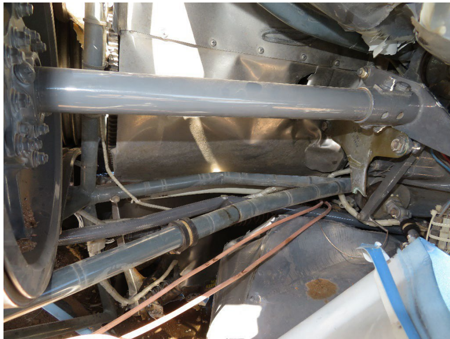
Photo of main rotor drive shaft (NTSB Photo)
